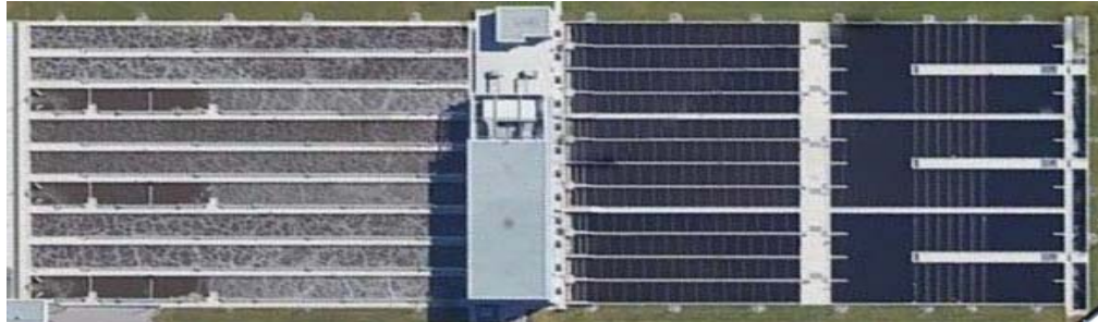
3-pass plug flow tank
