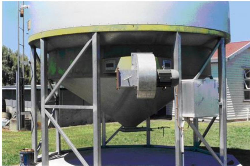
Fig 4. A Kotzur® Drying silo is one example of a silo designed for aeration drying. Fitted with a 7.5kW motor & fan combination capable of producing air flow rates of 10 - 20 L / sec /tonne.
