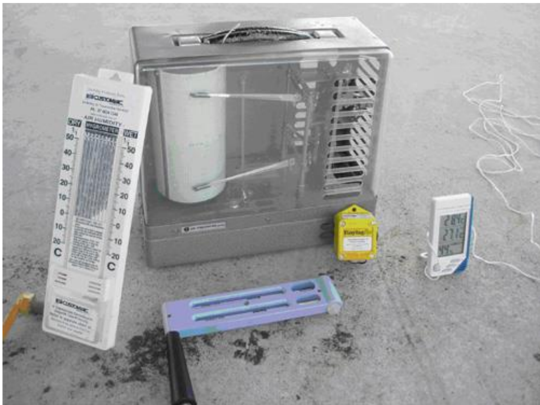
Fig 2. A range of equipment used to measure temperature and RH.
