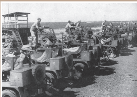
B-24 tail turret trainers mounted on trucks provide the student with the basic feel of what it will be like to operate the turret in the real aircraft.
