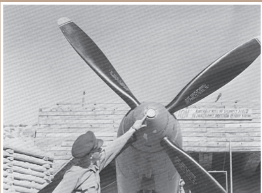
Red light in the prop spinner of this Bell P-63 would light up to show the student he had scored a hit.
