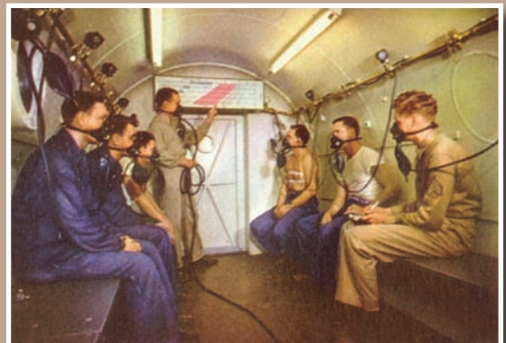
The Low Pressure Chamber took student gunners to the bombers operating altitudes without ever leaving the ground.
