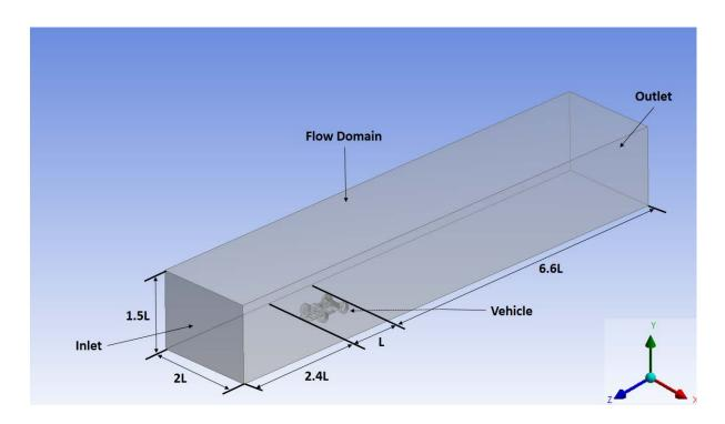
The mesh was generated using the integrated meshing tool available on ANSYS Workbench©. To improve the validity of the CFD results a mesh independence study was performed (Figure 5). Each mesh file used a default growth rate of 1.20. The final mesh file comprised of 933,024 elements with a minimum sizing of 4 mm to accurately model the complex geometry of the car (Figure 3).
