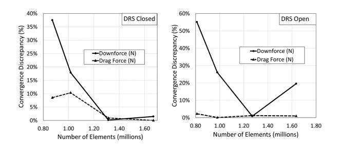
Although a higher level of convergence would be preferable for the downforce with the DRS open, limitations in computation power were causing excessively long computational time. However, as the primary focus of the DRS open configuration is the drag force, the results can be used as there was only a 1.0% discrepancy for this parameter.
