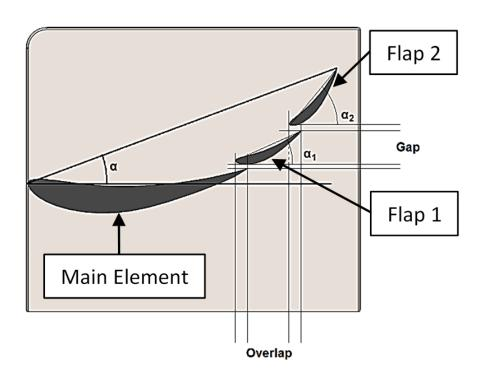
To achieve a highly efficient multiple-element design, many variables such as the angle of attack (AOA) of each element, gap and overlap need to be optimised for the specific requirements of the design. However, to produce a design in a suitable
