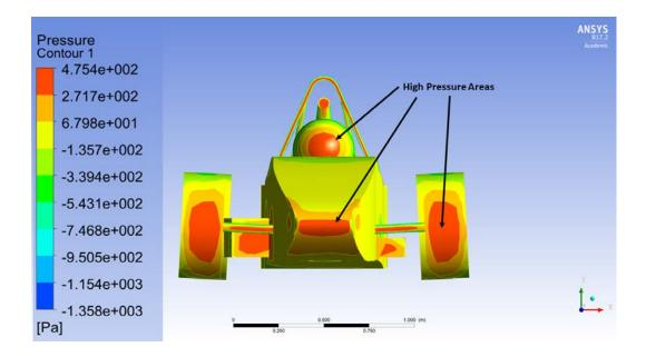
The coefficient of lift ( $C_L$ ) and coefficient of drag ( $C_D$ ) are dimensionless values which are used as an indication of a vehicle's aerodynamic performance. Using the force value acting on the vehicle in the Z axis of 277.6 N, the resulting  $C_D$  was calculated (Eq. 2).
