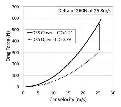
The resulting reduction in drag force was calculated to be 35% with the DRS open (Eq. 3).
