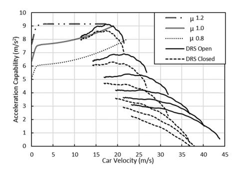
The acceleration potential increased by 15.7% at a velocity of 25 m/s with the DRS open. In an attempt to predict and compare the performance over the 75 m acceleration event, an online FSAE vehicle simulator (FSAESim.com) was used with the inputted vehicle characteristics. The simulator predicted a time of 5.31 s and the result for the 2017 Hungary event was 5.49 s, a similarity of 96.7%.
