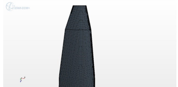
Fig.7. Blade surface grids in the tip region
