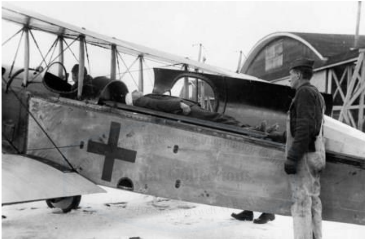
Figure 1 Curtiss JN-4 Used as an Air Ambulance. Reprinted from Skaarup, Harold A. "Canadian Warbirds 2: The Biplane Era, Trainers, Transports and Utility Aircraft." Military History Books. Accessed 18 October 2016. http://silverhawkauthor.com/canadian-warbirds-2-the-biplane-era-trainers-transport-and-utility-aircraft-book_309.html .
