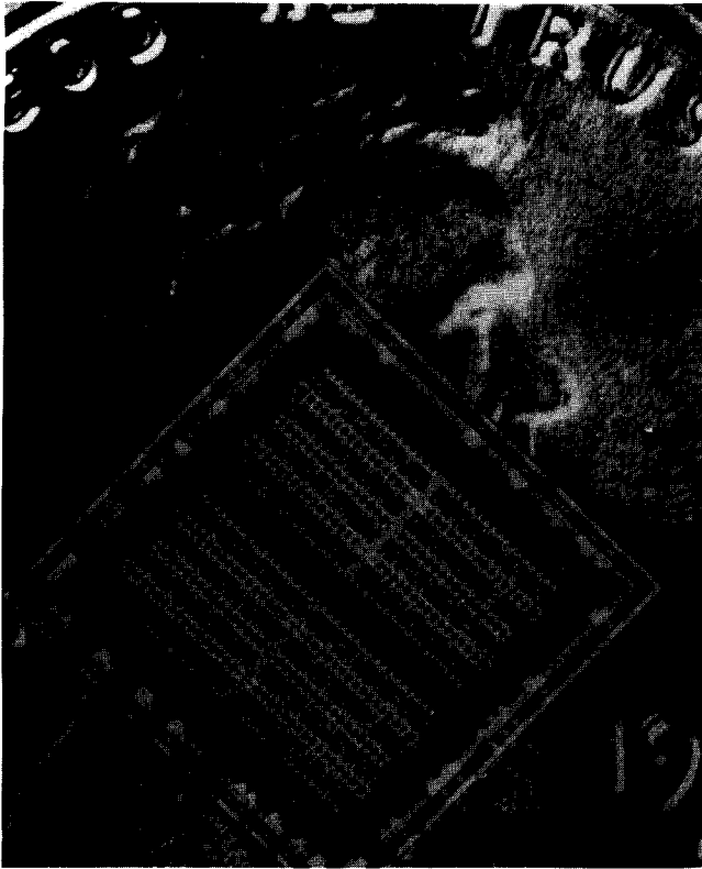
The VLSI (Very Large Scale Integrated) chip developed for operational use as part of the Hubble Space Telescope ground data system by the University of Idaho Center for Space Engineering Research, shown here on a penny to indicate scale.
