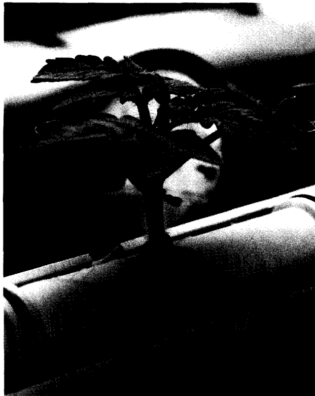
Close-up of tomato plant growing in a plant culture system designed for NASA. Two plastic pipes are fitted one inside the other. The inner pipe is wettable and porous. It serves as the source from which the roots draw nutrients and also helps support the roots. (USDA, Agricultural Research Service photo)
