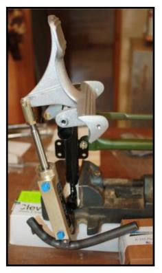
The photo on the left shows the master cylinder attached to the toe brake. The bottom end of the master cylinder attaches to a curved mounting bracket. The curved mounting bracket is welded to the airframe in accordance with SAR drawing 3-1536. SAR drawing 4-1624 provides details for installing these components.
