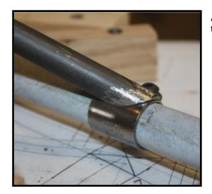
A hand grinder is used for final fitting of the tubes to the tube loops.
