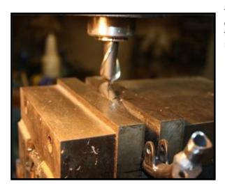
The milling machine vice was rotated 26 degrees and a round nose end mill was used to fit the rear end of the support bracket to the rear loop.
