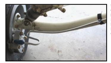
The aluminum hydraulic line provide with the kit is installed with an "S" bend located at the caliper as shown in the photo. The metal braided hydraulic line provided with the kit is installed on the top end of the lines to connect to the bulkhead fittings.
