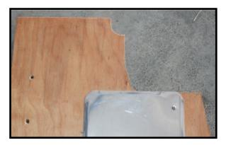
The front of the floorboards must be modified to provide clearance for the master cylinders.
