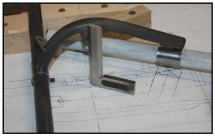
The left end of the bracket is trimmed to fit the profile of the loop and to properly position the bracket attachment tabs. For reference, the 1/2" tubing is .049" thick and the tube loops are .050" thick. The forward loops are positioned so that a bolt and nut can be inserted with the firewall positioned against the front side of tube 45. The aft loop is positioned at
