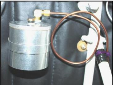
is mounted on the aircraft cabin side of the fire wall with the bottom of the reservoir higher than the top of the master cylinder inlets. There is a 1/8"copper overflow tube connected to the top of the reservoir. The copper tube is routed to the exterior of the aircraft. When the brakes are bled, brake fluid will fill the reservoir and overflow to the exterior of the aircraft.
