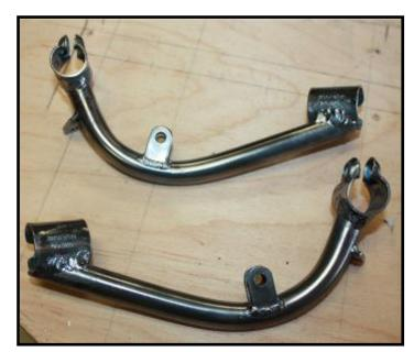
The loops are then finish welded to the brackets, and wire brushed to prepare for painting.
