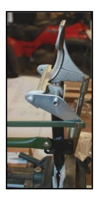
These photos show the right side front and rear rudder and toe brake pedals temporarily mounted for parts fitting.
