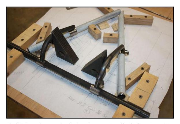
Wood blocks are then screwed to the plywood to accurately position the three tubes and four loops. The white tubes are 3/4" and the black tube is 5/8". The location of the loops are located from the pattern. Shim blocks are used to space the tubes equal distance from the base.
