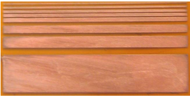
Figure 13. Demonstrator test pattern (Cu plated on PI) created by the catalyst-layer approach.
