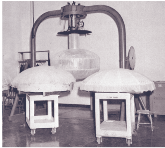
Figure 7. Early testing by Lockheed of candidate constructions of multilayer insulation (MLI).
