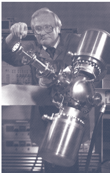
Figure 8. Hughes three-stage 12 K Vuilleumier cooler used dual opposed pistons.
