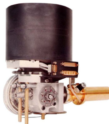
Figure 3. Hughes Aircraft two-stage Vuilleumier (VM) cooler flown on SESP 71-2 in October 1971.
