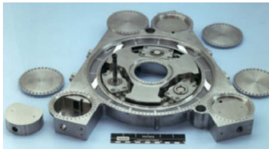
Figure 19. Hughes rotary magnetic cooler for cooling between 10K and 20K.
