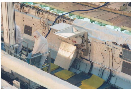
Figure 52. 10K BETSCE cryocooler integrated onto space shuttle STS-77.
