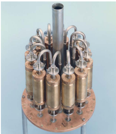
Figure 23. JPL 20 K Charcoal/H 2 sorption compressor of 1983.
