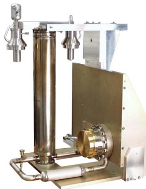
Figure 40. Creare NICMOS turbo-Brayton cryocooler flown on HST in 2002.
