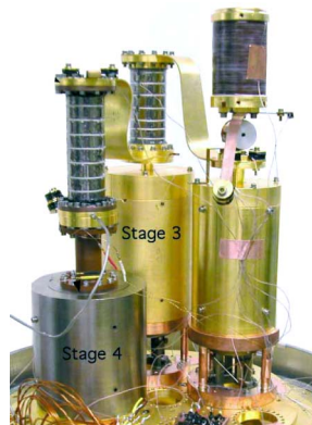
Figure 56. Sub-Kelvin ADR refrigerator for Constellation-X.
