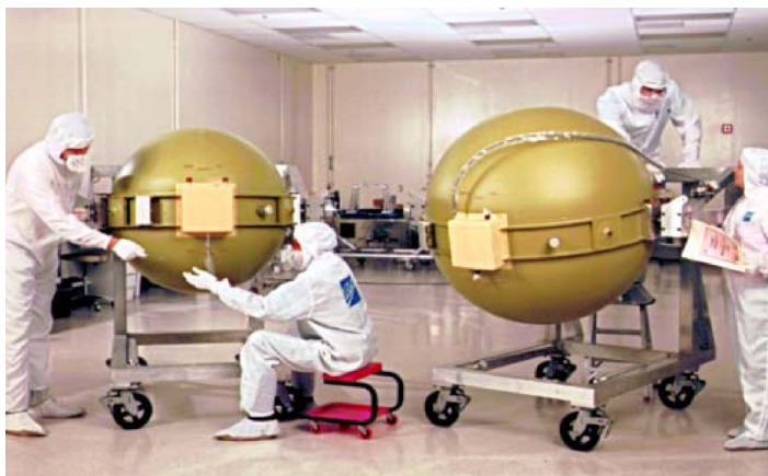
Figure 13. Over 60 of these Power Reactant Storage Assembly (PRSA) dewars were built by Beech Aircraft and Ball Aerospace to supply the Shuttle's fuel cells with hydrogen and oxygen.
