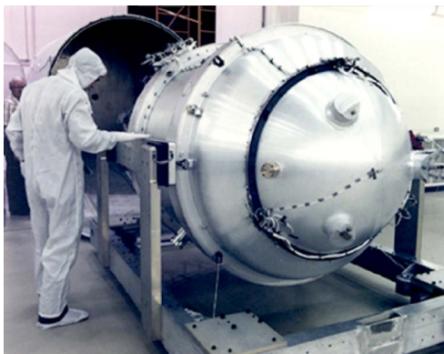
Figure 25. Ball Aerospace superfluid helium dewar used for COBE was derived from the IRAS dewar flown in 1983.
