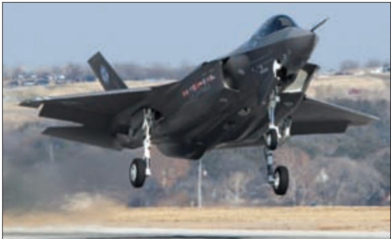
The Lockheed Martin F-35 Lightning II has the ability to take off and land vertically (STOV/L), or use an increase in the angle of attack in a conventional takeoff (CTOL). Image by Lockheed Martin.
