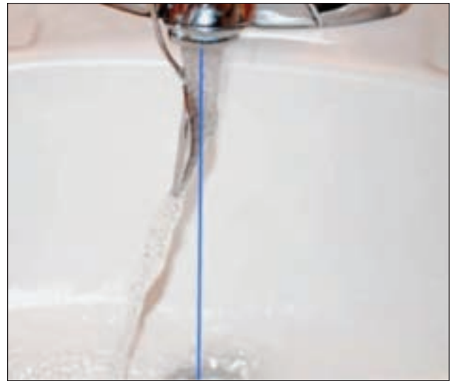
This demonstrates the Coanda effect. The blue line is the direction the water would flow normally. When the spoon is inserted into the flow, the water “sticks” to the spoon and bends toward the tip.
