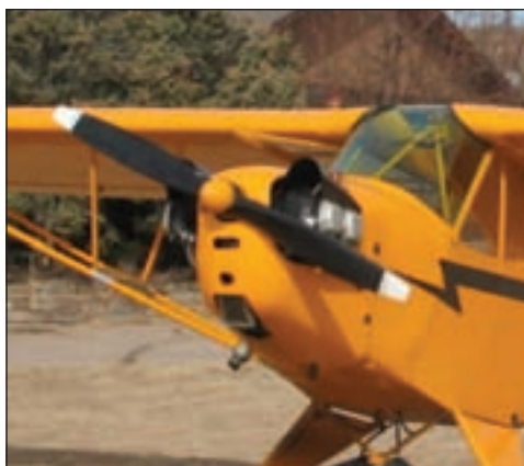
Starting at the hub, you can see how the blade changes in angle, chord, and area on this restored Piper Cub. Just like a wing, the rotating propeller harnesses the energy of the air and converts it to thrust.
