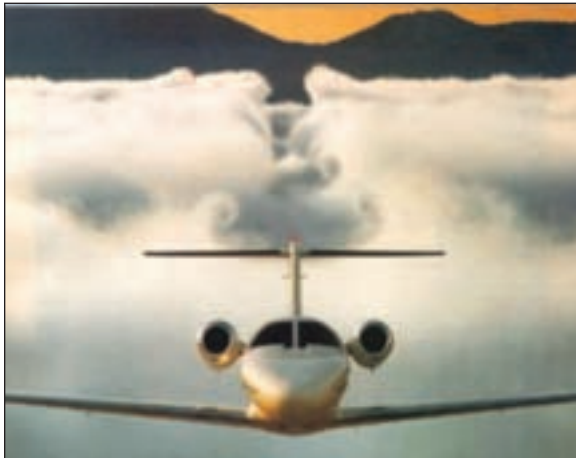
This picture dramatically shows airplane downwash. The Cessna Citation has just flown above a fog bank shown in the background. The downwash from the wing has pushed a trough into the cloud formation. The swirling flow from wingtip vortices is also evident. The picture was taken by Paul Bowens and the image was provided courtesy of Cessna Airplane Company.
