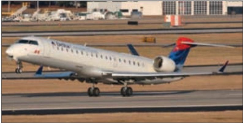
The pilot of this Canadair CRJ-700 has increased the angle of attack prior to takeoff. Angle of attack is also increased just before landing to slow the aircraft and provide an additional amount of control at low speed. Image courtesy of Adam Wright, First Officer, Atlantic Southeast Airlines.
