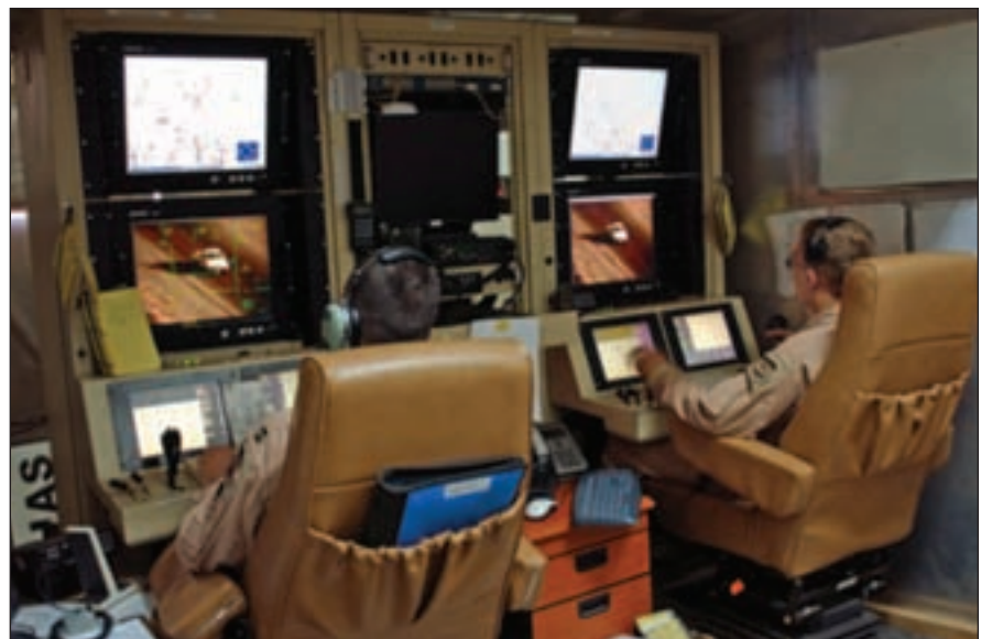
A ground control station crew performs post takeoff checks after launching an earlier Predator MQ-1 from Ballad Air Base in Iraq. USAF image by Master Sergeant Steve Horton
