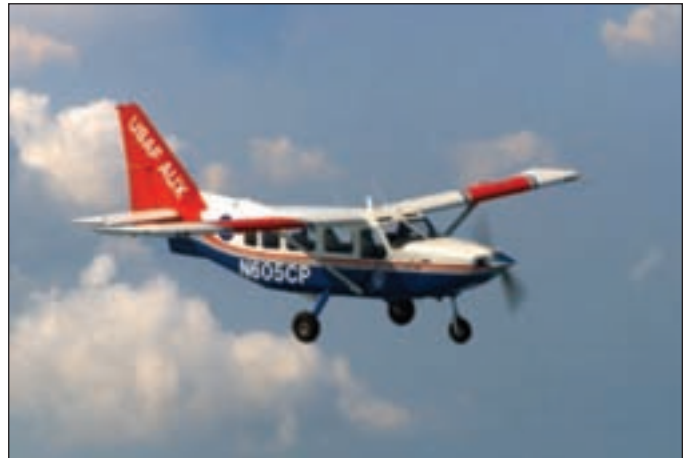
This is the Civil Air Patrol Gipsland GA-8. When you look at this photograph, imagine what the plane is doing to the surrounding air. As the air passing over the wing speeds up, it passes behind the wing and creates a downwash. This puts a force against ALL of the air surrounding the wing ... and the airplane flies.
