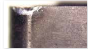
Kennametal's CNGG-432FS KC5510 Tool life: 26.5 minutes
