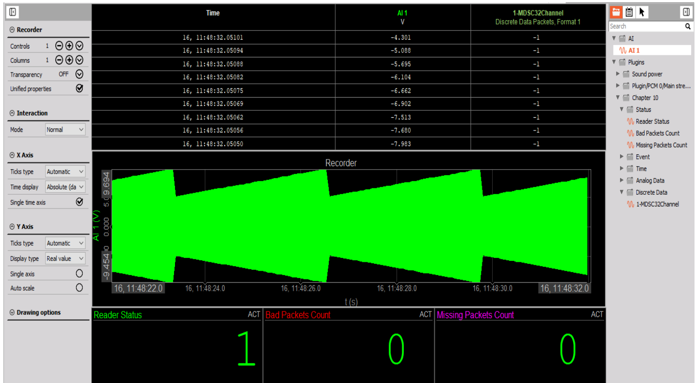
Image 76: To visualize wanted channels on the display, click on the names of channels on the right panel
