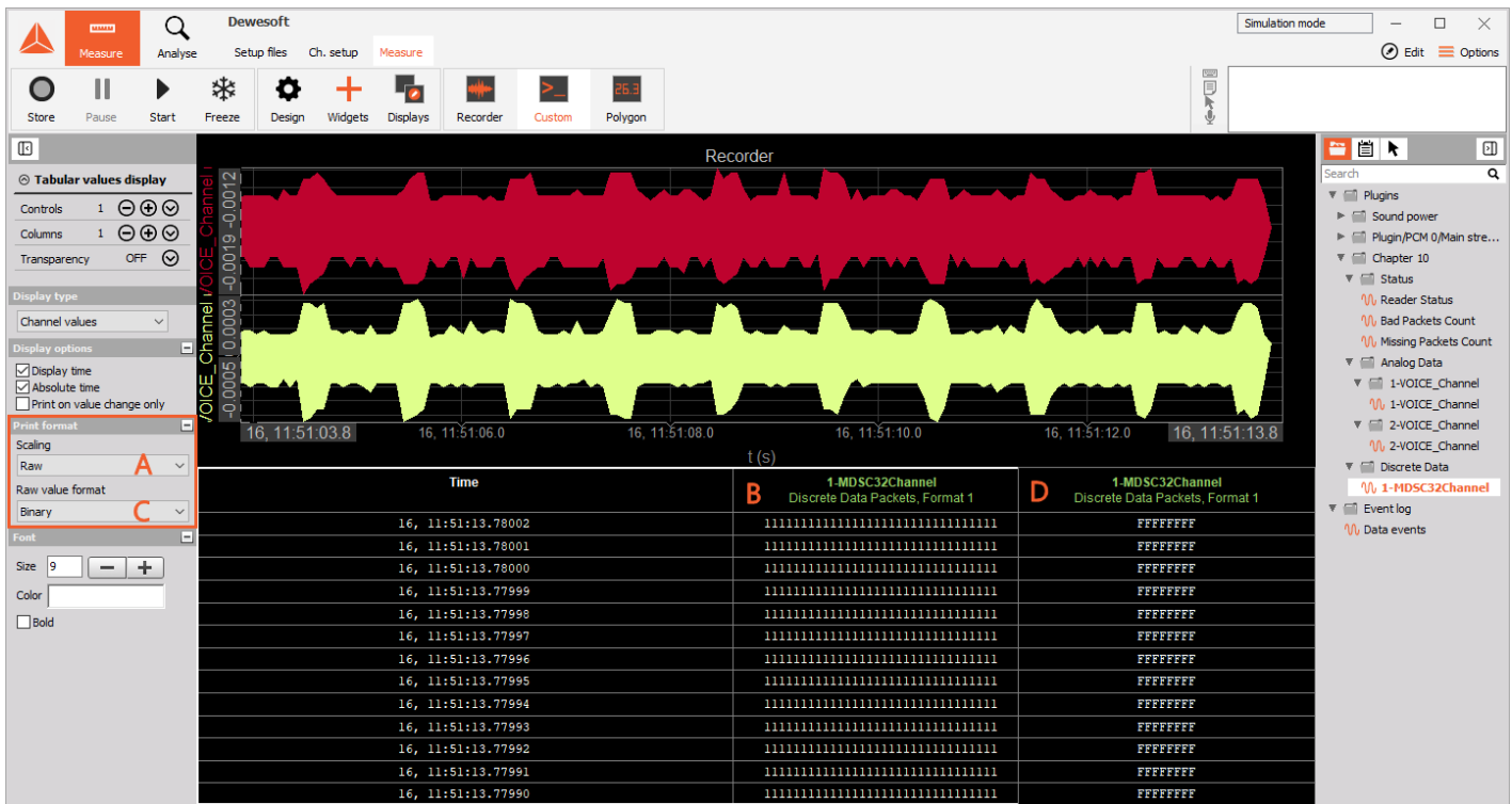
Image 65: Add recorder, tabular values display and apply channels to them
