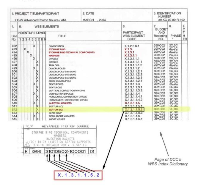
**Figure 9–2:** Breakdown description of a WBS number for a component in the ring. The first '1' refers to construction phase and is ignored.
