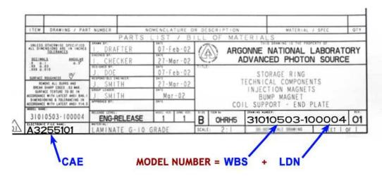
**Figure 9–1:** Title block of a typical APS engineering drawing. CAE, WBS, and LDN numbers are shown. The "drawing number" is a hyphenated combination of the WBS and LDN.
