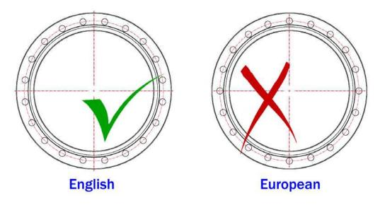
**Figure 8–1:** Proper orientation for aligning flanges (to be followed unless spatial interference conditions exist).
