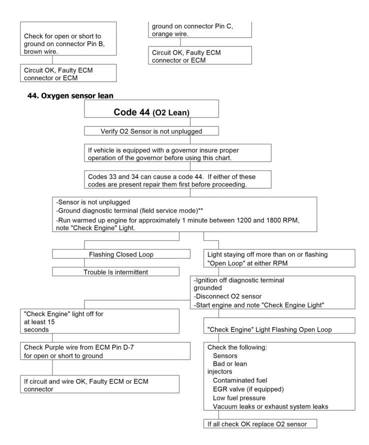
\*\* Service diagnostic mode is entered the same as Engine Off Self Test. Ground out Pin A and B on the ALDL connector with the engine running. Rapid flashing (approx 1/2 - 1 sec interval) is open loop. Flashing at a slower rate indicates closed loop.
