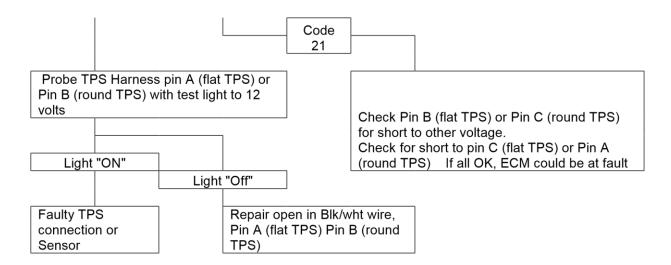
22. Low voltage at throttle position sensor
