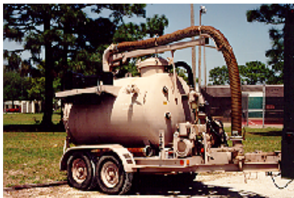
Figure 13. Wastewater Disposal Trailer.
