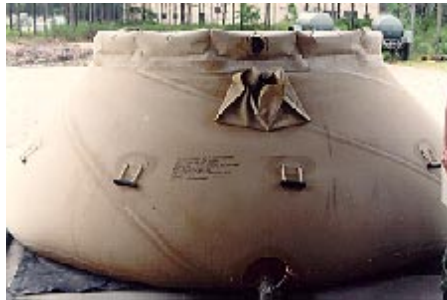
Figure 12. 3000-Gallon Water Storage Tank.
