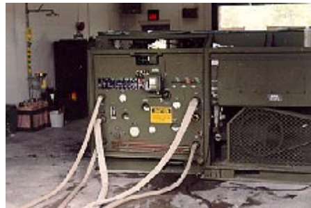
Figure 7. Reverse Osmosis Water Purification Unit.
