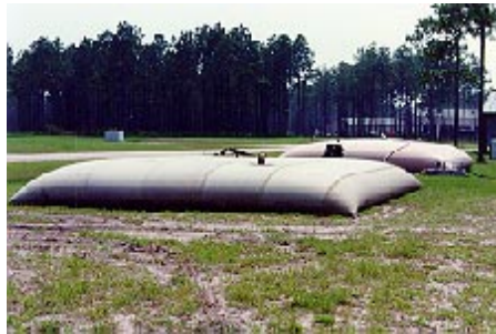
Figure 11. Water Storage Bladder.
