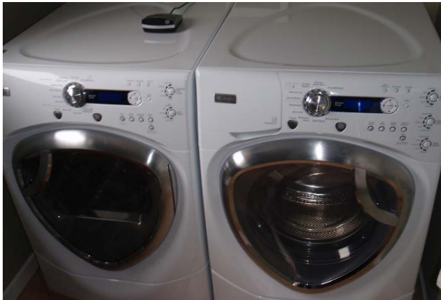
Antenna for data exchange with GE/Silver Springs meter on the other side of the wall
