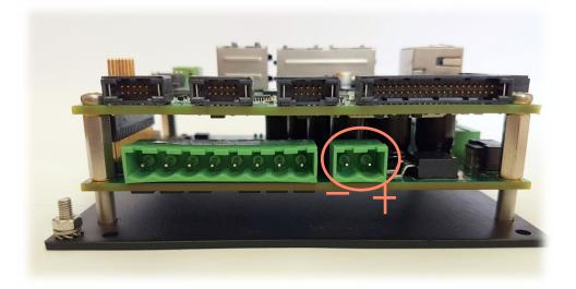
Manufacturer: P/N (product side): Pitch: DEGSON (Phoenix compatible) 2EDGRC5.0802P14H 5.08mm
