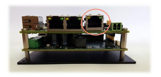
Description: Cable: RJ45 LAN 10/100Base-T Connector with magnetic CAT5
