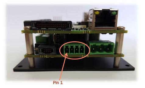
Manufacturer: P/N (product side): Pitch: DEGSON (Phoenix compatible) 15EDGRC3.504P1400AH 3.5mm
