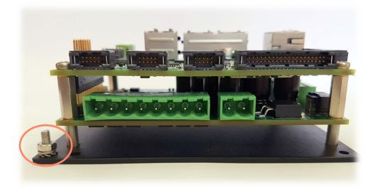
The chassis, within the product, is not connected to the power supply ground.
