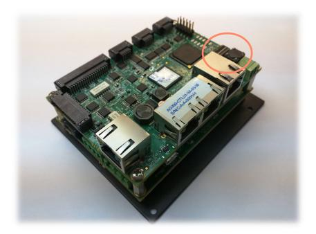
The DIP switches have few purposes, such as defining the address offset of the unit over a CAN Bus daisy chain connection or Ethernet IP value and also some other internal purposes, all as described in the following table.
