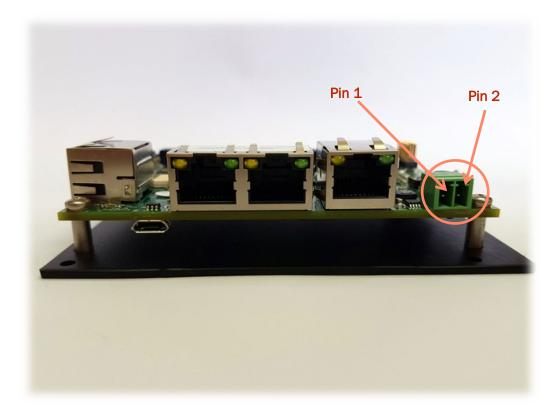
Manufacturer: P/N (product side): Pitch: DEGSON (Phoenix compatible) 15EDGRC3.502P1400AH 3.5mm
