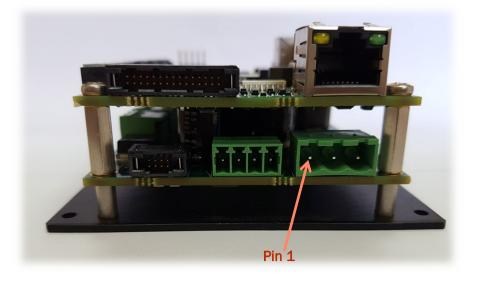
Manufacturer: P/N (product side): Pitch: DEGSON (Phoenix compatible) 2EDGRC5.0803P14H 5.08mm
