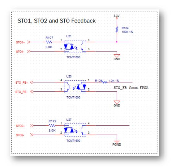
The electrical characteristics of the STO1 and STO2 inputs are identical to those of the discrete, isolated inputs of the controller. Refer to the chapter about J9 above.
