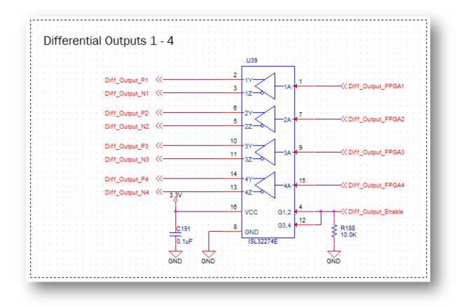
The differential outputs are disabled immediately after power on, till they are controlled by the software and the user defined parameters.
