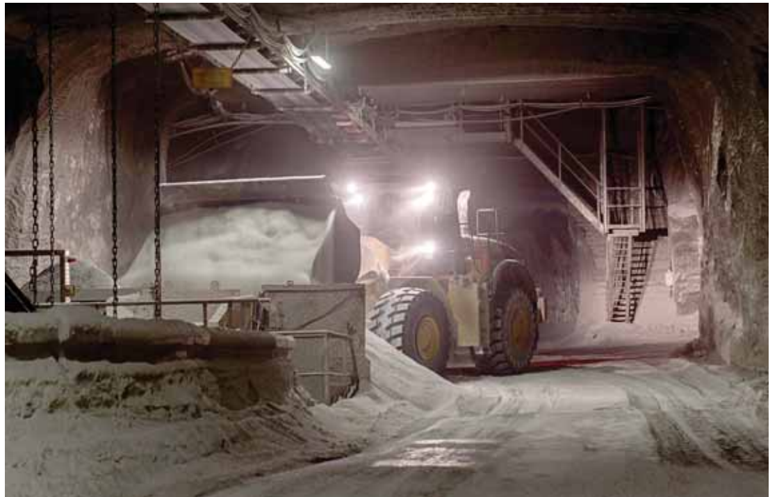
A wheeled digger dumps a shovelful of salt onto a conveyer inside the Stetten Salt Mine in Germany.
