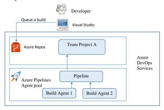
The preceding diagram is a typical set up on how to build an Azure Pipelines and recommended for AB Suite. Each pipeline agent that hosts the Build Agents requires a full install of the AB Suite Developer and SQL Server software. This part will guide you through the required settings to allow Visual Studio build definitions to work with AB Suite projects. The build agent can be installed on a local machine or an Azure VM.
