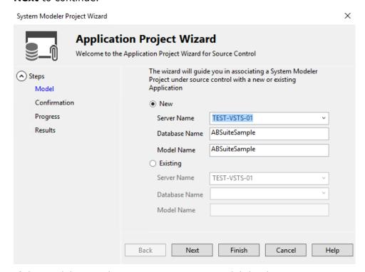
If the model size is large, creating a new model database is going to consume time. You can clone an existing model database and then connect it by selecting **Existing**.
