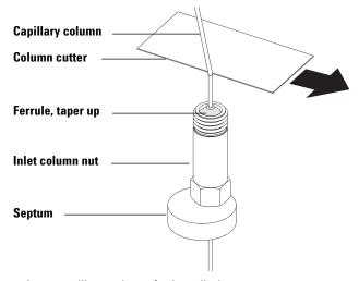
Figure 3 Preparing a capillary column for installation
