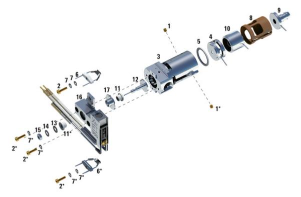
Figure 14 Disassembling the extractor El ion source
