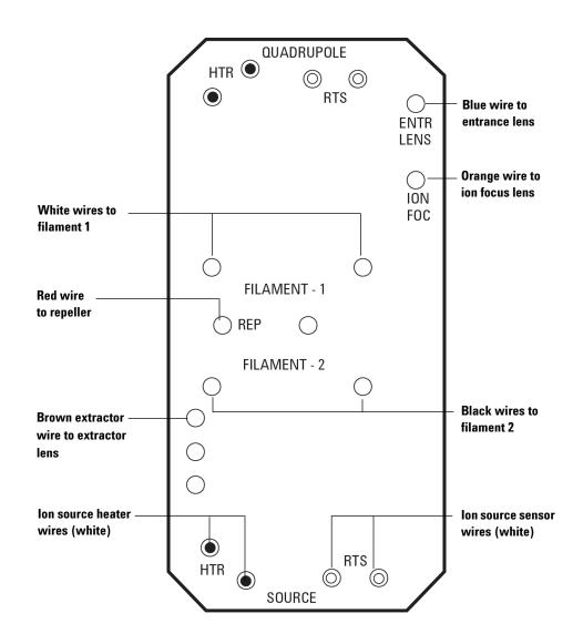
Figure 20 Feedthrough board wiring
