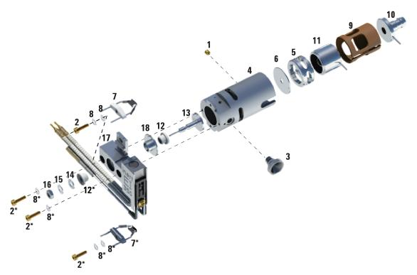
Figure 13 Disassembling the standard or inert El ion source
