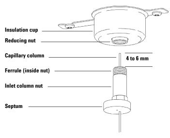
7 Position the column so it extends 4 to 6 mm past the end of the ferrule (Figure 4).
