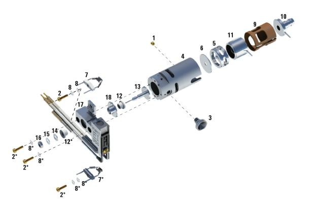
Figure 16 Assembling the standard or inert El ion source
