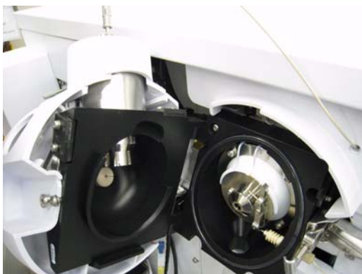
Figure 24 Opened spray chamber
