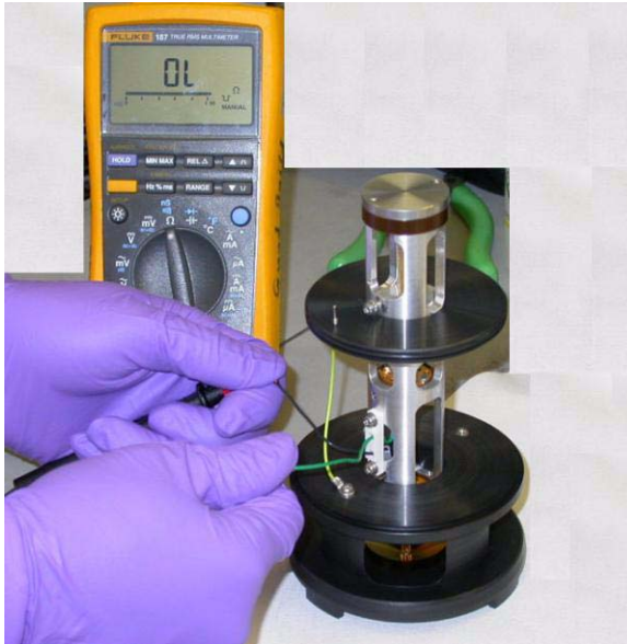
Figure 62 Testing for continuity.
