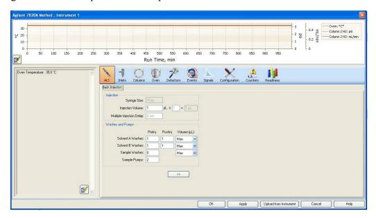
• Clicking the Inlets button opens the options to configure the inlet temperatures and flow rates. **NOTE**: Make sure the "heater" and "pressure" boxes are checked in both the front and back inlet windows. Standard conditions include inlet temperatures @ 250-300 °C and a flow rate of 100 mL/min @ 100:1 split. To conserve gases, the inlet that is not being used for the method should be set to a splitless flow of 15 mL/min.
