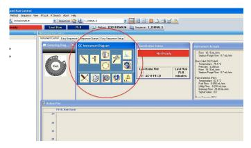
• Clicking on the ALS button on the top of the GC Instrument window opens the options to configure the auto-sampler. Standard parameters are shown below:
