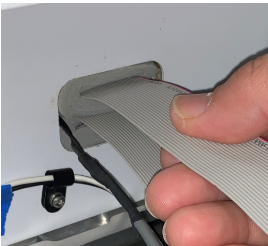
Figure 10 Pulling excess cable from enclosure formed when inserting the foam sandwich
