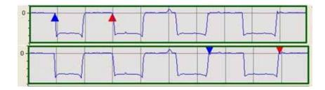
Figure 99 Cross section in Y direction showing non-linearity
