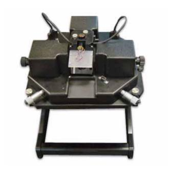
Figure 11 5500 SPM microscope on support stand
