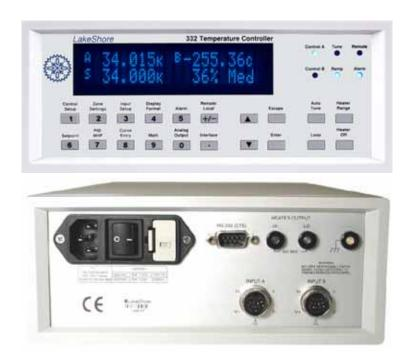
Figure 127 Lakeshore temperature controller
