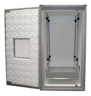
Figure 23 Vibration isolation chamber
