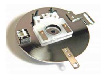
Figure 124 Liquid cell mounted on standard sample plate
