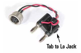
Figure 132 Tab side of Cable 3 must be inserted into the Lo jack.
