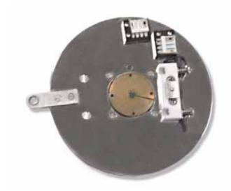
Figure 133 Peltier (Cold MAC) sample plate.
