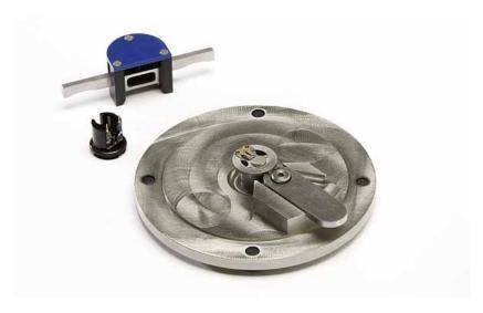
**Figure 40** Two-piece nose assembly, removal tool and assembly jig. The nose assembly disk is shown on the jig; the body is shown to its left.
