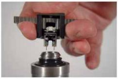
Figure 34 Using the nose assembly removal tool
