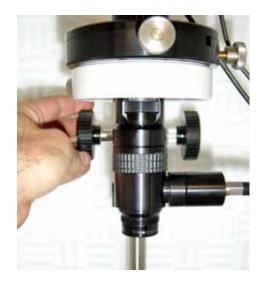
Figure 59 Adjusting the z-position
