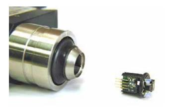
Figure 84 CSAFM nose assembly and scanner
