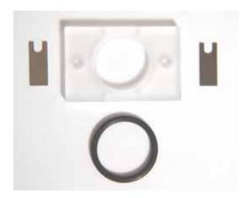
Figure 123 Liquid cell components
