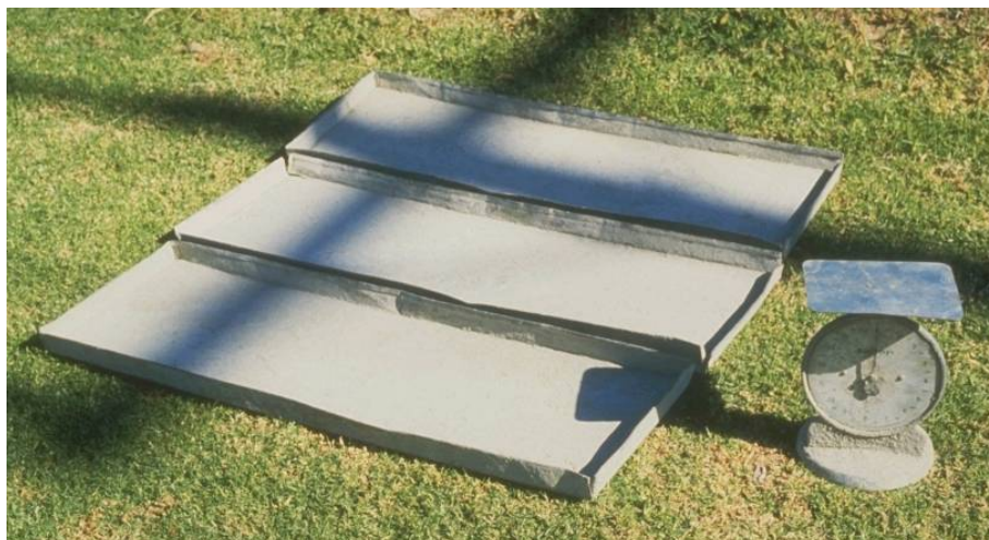
Figure 7.4 Use of trays to verify the binder application rate
