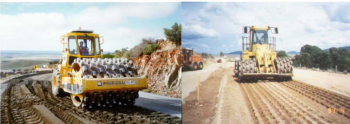
Figure 7.15: Static padfoot (left) vibrating padfoot (right) compactors
