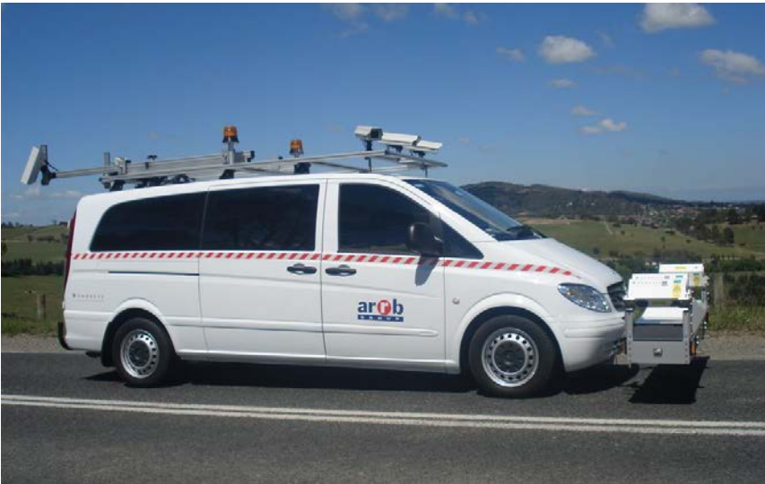
Figure 6.6: Survey vehicle featuring laser profilometer to measure ride quality
