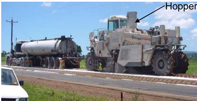
Figure 7.2: A reclaimer with an integrated powder binder hopper and load cells
