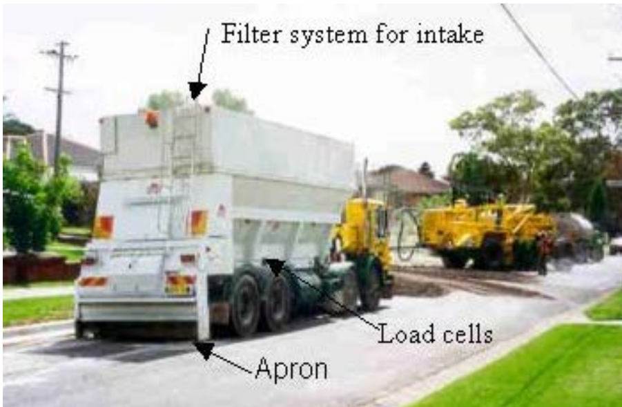
Figure 7.6: Desirable features of a mechanical spreader
