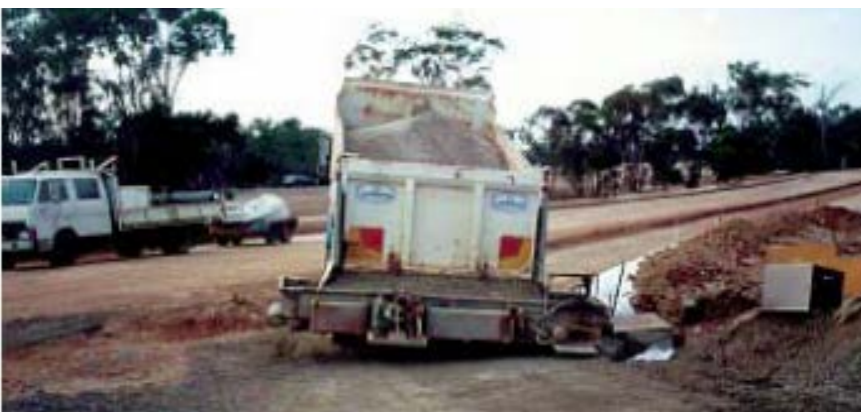
Figure 5.2: Horizontal discharge unit
