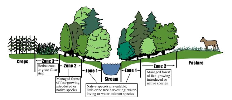
Figure 3. Buffer Strip Function
