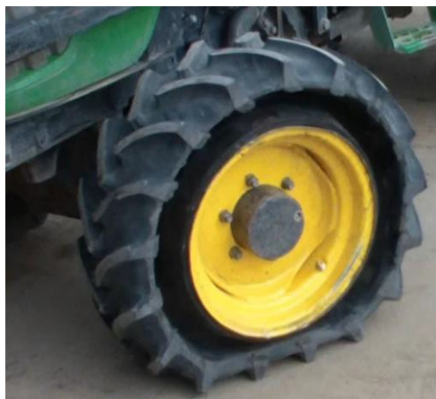
Figure 22. Galileo wheel with accordion-shape sidewall design. 78
