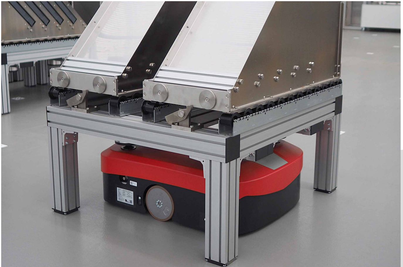
Low-platform vehicle with load-bearing frame made from an aluminium profile with customer-specific product carriers
