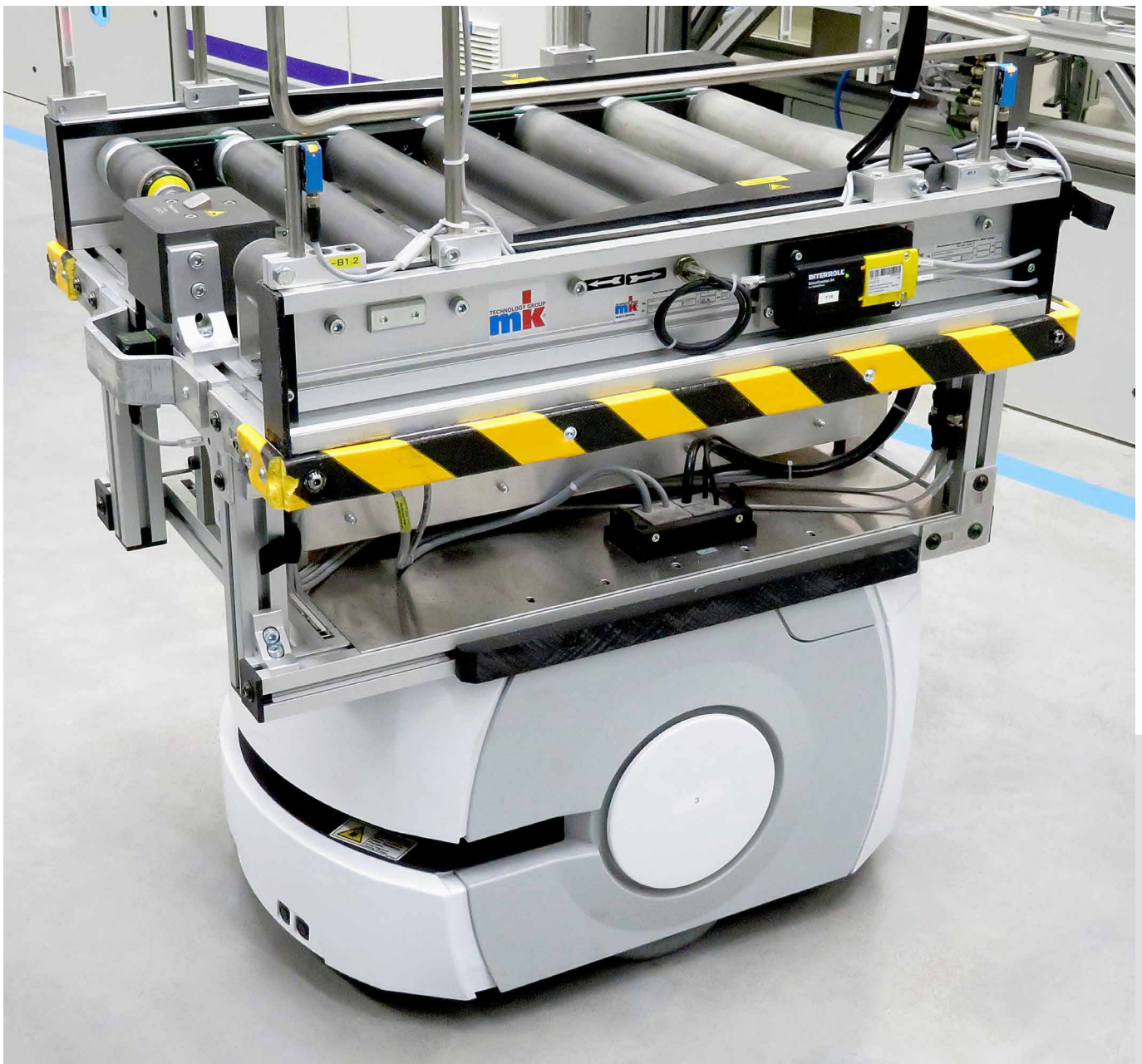
Piggyback vehicle with customised load carrier for transporting small load carriers
