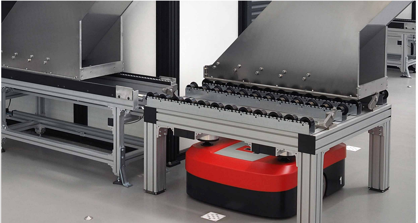
AGV to transfer station: A magnet pulls the specimens from the frame via a gravity roller conveyor
