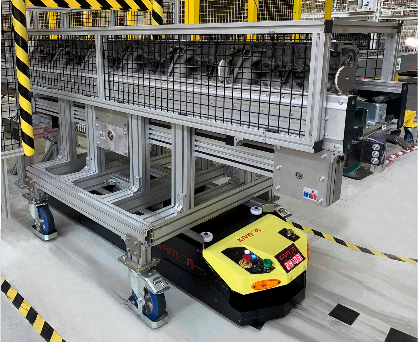
Low-platform vehicle with trolley made from an aluminium profile incl. actuated roller conveyor and protective device guard at transfer station
