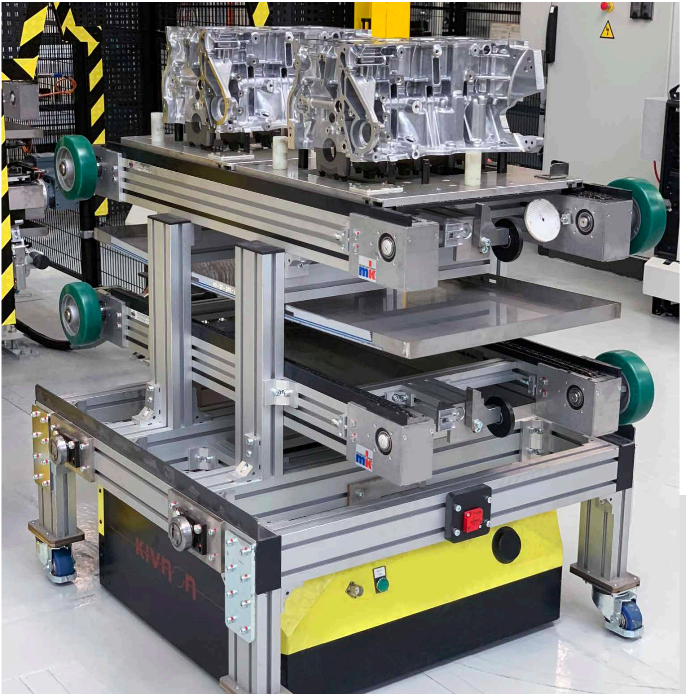
Low-platform vehicle with mobile profile frame and chain conveyor driven by friction wheels
