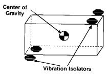
Diagonal Center-of-Gravity Installation
