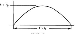
FIGURE 23 FORCE-TIME CURVE—RESPONSE THROUGH SHOCK MOUNTS SHOCK REDUCTION
