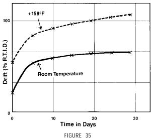
TYPICAL DRIFT CURVE—SPE® I ELASTOMER (30 PSI)
