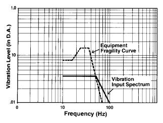
FIGURE 14 EQUIPMENT FRAGILITY VS. VIBRATION INPUT
