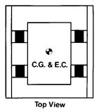
FIGURE 28 SIMPLE SHEAR MOUNTING SYSTEM
