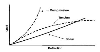
FIGURE 15 LOAD-DEFLECTION CURVES FOR "SANDWICH" MOUNTS
