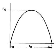
FIGURE 22 FORCE-TIME CURVE—INPUT TO CONTAINER
