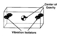
Horizontal Center-of-Gravity Installation
