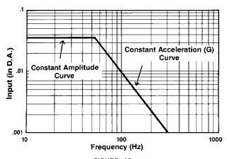
FIGURE 12 COMPARISON-CONSTANT AMPLITUDE TO CONSTANT "G" VIBRATION INPUT
