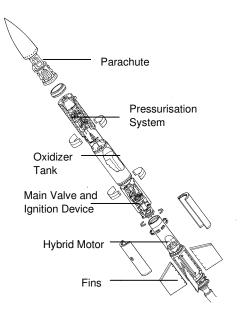
Figure 2: Final Configuration of HERA
