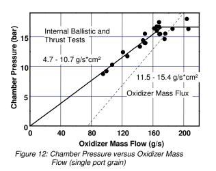
Therefore the average oxidizer mass flux of the rocket was set to 9 g/s\*cm<sup>2</sup>. The expected average chamber pressure for a single port configuration without mixing devices for 170 g/s is 16.5 bar. Firings with the HERA motor testbed confirmed this expected value.
