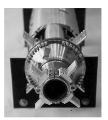
Figure 3: Nozzle Assembly of Rocket
