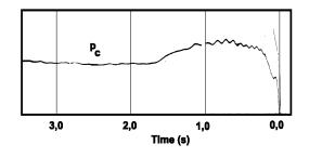
Figure 13: Chamber Pressure versus Time Test (Internal Ballistic Test)
