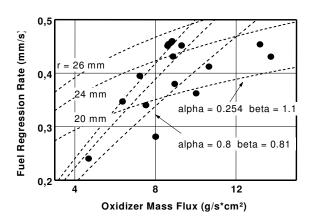
Figure 19: Fuel Regression Rate versus Oxidizer Mass Flux
