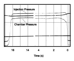
Figure 15: Typical Smooth Internal Ballistic Test
