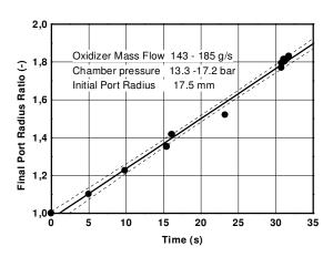
Figure 20: Final Port Radius Ratio versus Time
