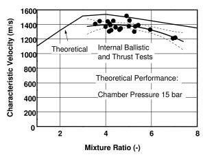
Figure 17: Experimental & Theoretical Characteristic Velocity versus Mixture Ratio
