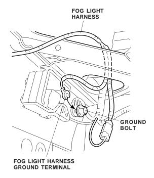
12. Secure the fog light harness 1-pin connector and the fog light harness to the vehicle harness with one wire tie. Do not secure the 1-pin connector to the SRS harness with the wire tie.
