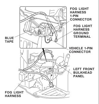
Locate the 1-pin connector blue-taped to the vehicle harness and remove the blue tape to free the 1-pin connector. Connect the 1-pin connector you just freed to the fog light harness 1-pin connector. 11. Loosen the ground bolt that fastens the vehicle ground terminal and secure the fog light harness ground terminal using this ground bolt.
