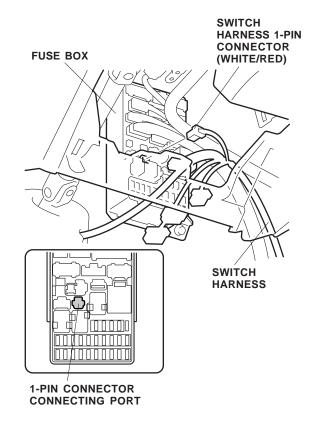
29. On A/T only: Unplug the vehicle 6-pin connector from the fuse box. Remove and discard the dummy connector from the 6-pin connector black-taped to the switch harness. Plug the switch harness 6-pin connectors in between the fuse box and the vehicle connector.
