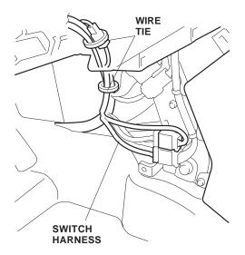
40. Plug the switch harness 5-pin connector (blue) into the switch, then install the switch in the hole in the instrument panel.
