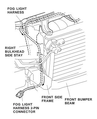
16. Align the green tape on the fog light harness (closest to the connector) with the hole in the front lower cross member, then secure the harness to the hole with the wire tie in the area shown.
