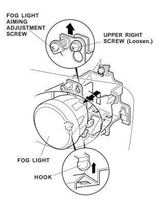
2. Remove the fog light connectors from the bracket stay, then unplug the connectors. Remove the fog light.
