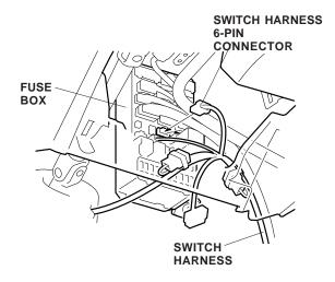
31. Unplug the vehicle 12-pin connector from the fuse box and plug the switch harness 12-pin connectors in between the fuse box and the vehicle connector.
