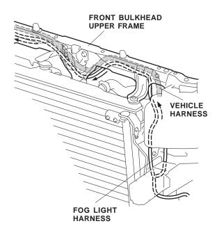
15. Continue routing the fog light harness 2-pin connector forward, then down to the bottom of the front side frame along the outside of the right bulkhead side stay.
