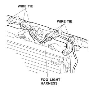
Secure the fog light harness to the holes in the bulkhead side stay and the side frame with four wire ties with clip.
