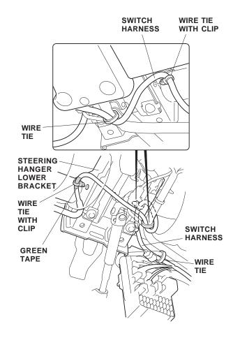
38. Secure the switch harness to the vehicle harness and to the hole in the steering hanger lower bracket with two wire ties and one wire tie with clip. Move the steering wheel up and down to confirm that the switch harness is not being pulled. Readjust if necessary.
