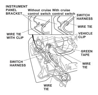
37. Attach a wire tie with clip to the switch harness at the green tape, then push the clip into the hole in the steering hanger lower bracket.
