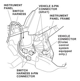
26. Slide the switch harness 8-pin connector onto the holder on the vehicle 8-pin connector (gray).
