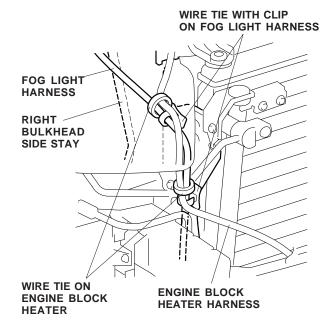
18. Secure the fog light harness to the vehicle harness with six wire ties in the areas shown.
