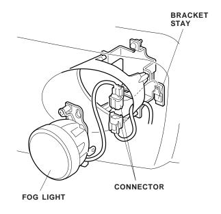
B. Remove the fog light rear cover (five screws).
