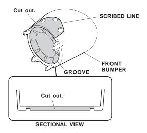
7. Inside the front bumper, slide the fog light into the cutout you made, and secure it with four self-tapping screws.
