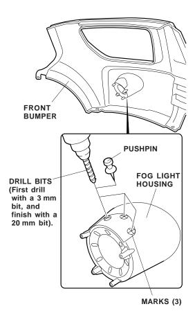
6. While being careful not to scratch the bumper, use a hacksaw blade to cut out the marked area from the front bumper along the inside of the scribed line and the groove on the back. Remove all burrs from the edges of the cutout.
