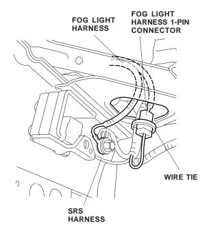
13. Behind the front side frame, route the fog light harness 2-pin connector (short end) down, and out through the clearance between the side frame and front bumper beam. Attach the wire tie with clip to the fog light harness at the green tape, then push the clip into the hole in the side frame.
