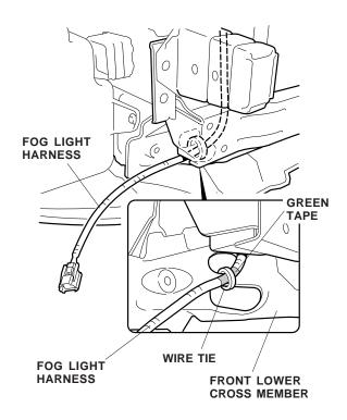
17. Attach the three wire ties with clips to the fog light harness at the green tapes, then push the clips into the holes in the bulkhead side stay. Further secure the fog light harness to the vehicle harness with two wire ties in the areas shown.
