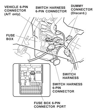
30. On **M/T** only: Plug the switch harness 6-pin connector into the fuse box.
