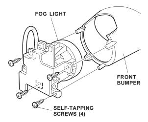
Repeat steps 5 thru 7 to cut the bumper and install the fog light on the right side of the bumper.
