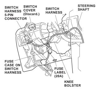
34. Remove the switch cover from the instrument panel, and pull the switch harness 5-pin connector out through the hole.
