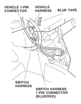
28. At the fuse box, plug the switch harness 1-pin connector (white/red) into the fuse box in the location shown.
