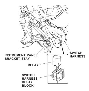
36. Align the green tape on the switch harness with the vehicle harness clip, then secure the switch harness to the vehicle harness with the three wire ties in the areas shown.
