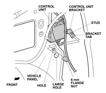
26. Install the back-up sensor harness clip into the hole in the vehicle panel.
