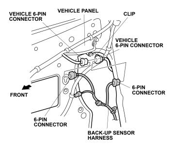
Plug the back-up sensor 6-pin connector into the vehicle 6-pin connector. Plug the other vehicle 6-pin connector into the other back-up sensor harness 6pin connector. 19. Reinstall the vehicle 6-pin connector clip to the vehicle panel.
