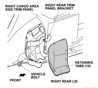
Remove the rear door and tailgate weatherstrip from the right cargo area side and two clips from the trim panel.
