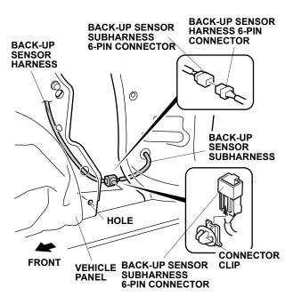
39. Plug the back-up sensor subharness 6-pin connector into the back-up sensor harness 6-pin connector, and install the connector clip. Secure the clip in the vehicle panel hole in the area shown.
