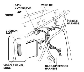
21. Using isopropyl alcohol on a shop towel, thoroughly clean the area where the cushion tape will attach. Attach the cushion tape to the edge of the vehicle panel at the location shown.
