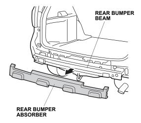
48. Using a utility knife, cut the rear bumper absorber along the preset line at the location shown.
