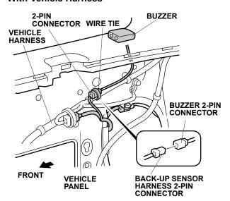
34. Secure the 2-pin connector to the vehicle harness with one wire tie (without vehicle harness: wire tie with clip B).
