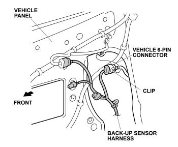
Secure the other 6-pin connector to the vehicle harness with one wire tie.
