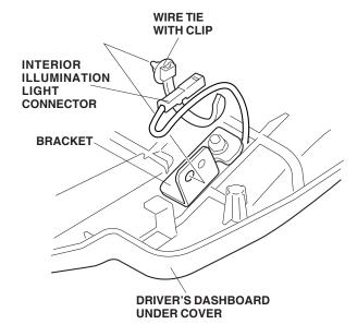
33. Reinstall the insulator to the driver's dashboard under cover, and pass the interior illumination light connector through the slit.
