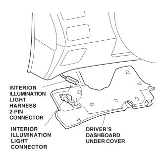
56. Plug the interior illumination light harness 2-pin connector to the interior illumination light connector on the lid of the dashboard center lower cover, and reinstall the lid.
