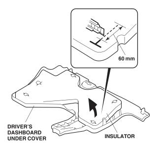
27. Secure template (A) to the driver's dashboard under cover with tape by aligning it with the square hole at the end of the curve as shown.
