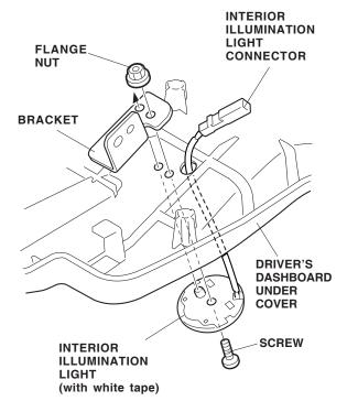
32. Bundle the interior light harness and secure the connector to the bracket using a wire tie with clip.
