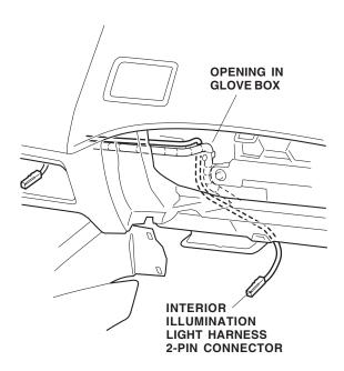
22. Secure the interior illumination light harness to the vehicle harness with two wire ties.
