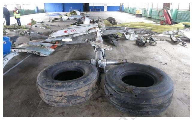
Fig. 9. The elements of the right main landing gear leg
