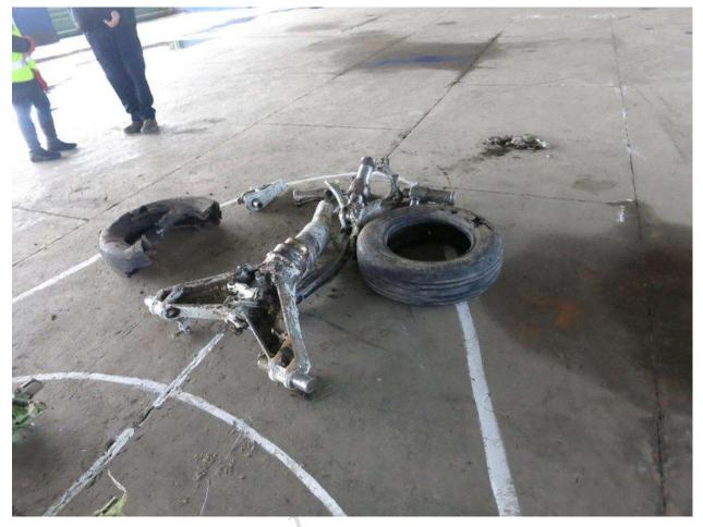
Fig. 8. Nose landing gear
