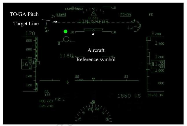
Fig. 56. The HUD reconstructed image at the point of time of 22:42:08.5
