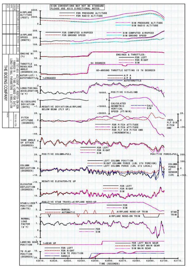
Fig. 46. The results of the engineering simulation (the pitch channel)
