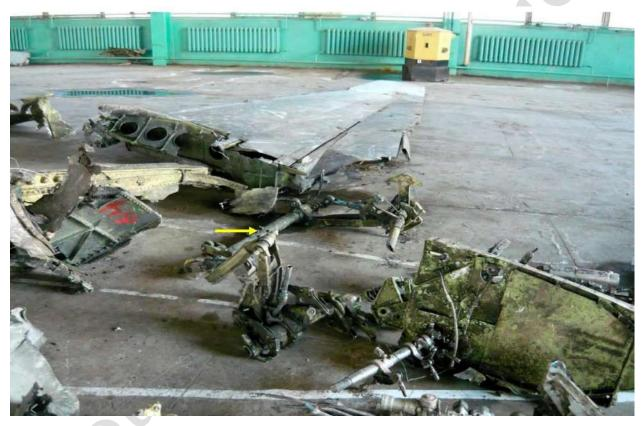
Fig. 11. The elevator control system output shaft (pointed with arrow)
