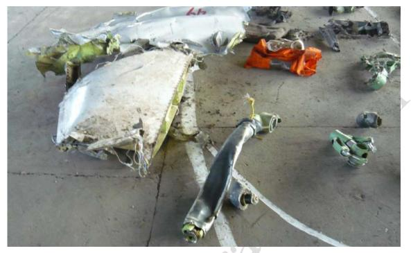
Fig. 2. The element of the F/O control column
