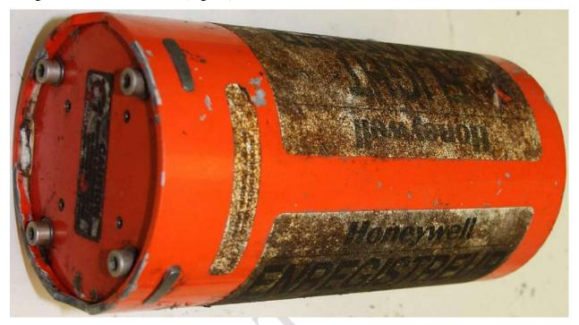
Fig. 35. The FDR secure memory unit
