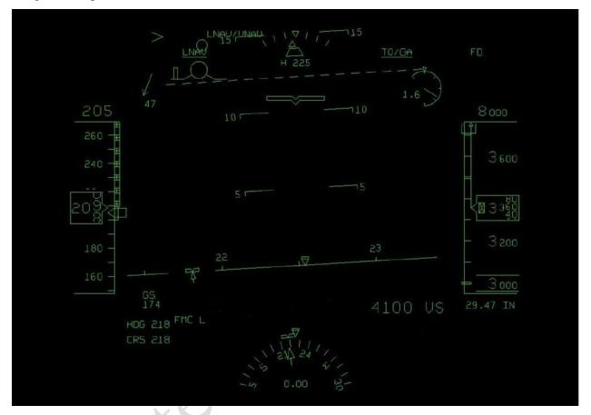
Fig. 69. The HUD reconstructed image at the point of time of 00:41:30.5 (the initiation of the stabilizer trim to nose-down)
