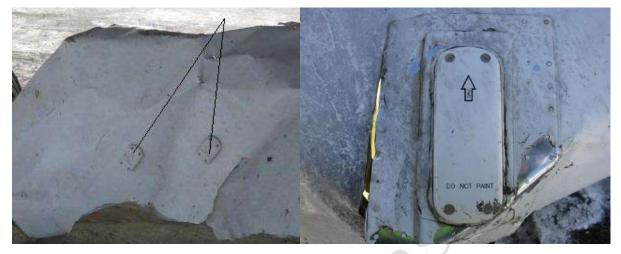
Fig. 26. The GPS and TCAS antennas
