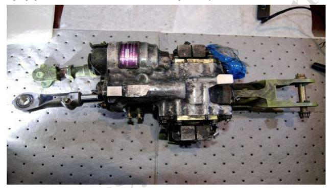
Fig. 45. The external view of the right PCU
