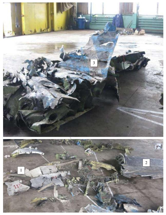
Fig. 7. The vertical and horizontal stabilizer elements (1 – LH half of the stabilizer, 2 - RH half of the stabilizer, 3- the vertical stabilizer elements)
