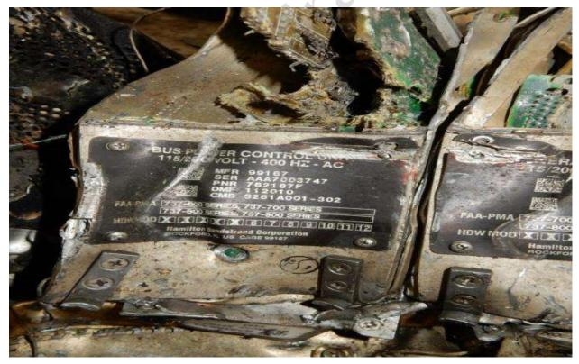
Fig. 21. The bus power control unit No 1
