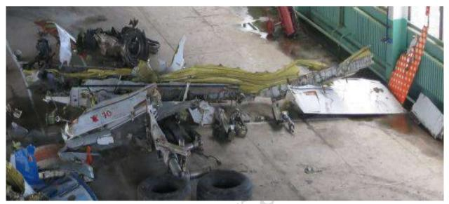
Fig. 4. The fragments of the RH wing panel
