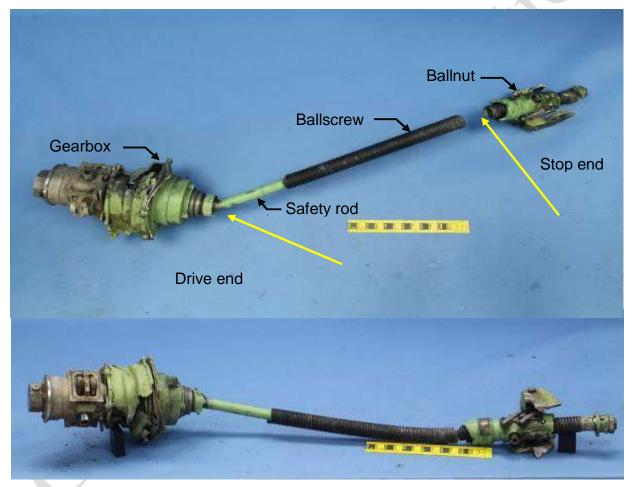
**Fig. 42.** The jackscrew assembly with the fractures (the fractures are pointed with arrows) At the outcome of the examination the following was established:
