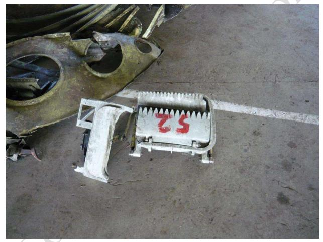
Fig. 13. The air conditioning system outflow valve
