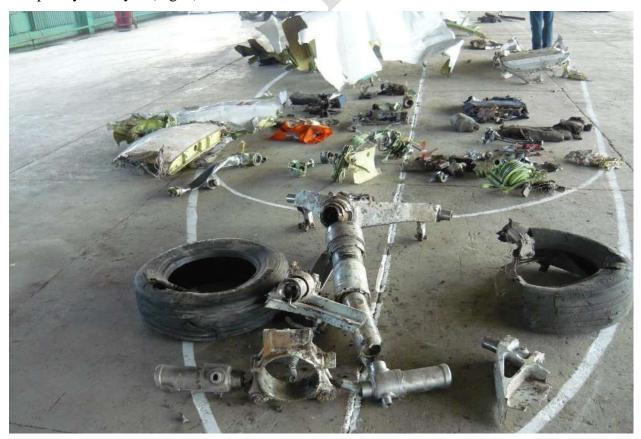
Fig. 1. The elements of the cockpit and the nose landing gear leg
