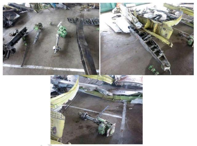
Fig. 6. Jackscrews and single unit tracks
