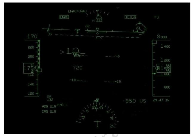
Fig. 64. The HUD reconstructed image at the point of time of 00:40:50 (the TO/GA mode activation)
