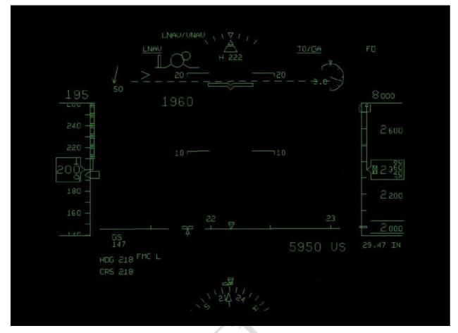
Fig. 67. The HUD reconstructed image at the point of time of 00:41:13 (the pitch local maximum ≈18.5°)
