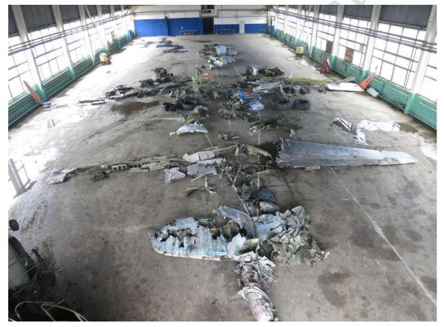
Fig. 41. The surface layout of the wreckage in the hangar
