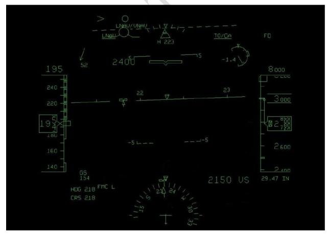
Fig. 68. The HUD reconstructed image at the point of time of 00:41:19 (the pitch command bar local maximum ≈13°)
