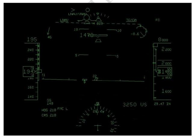
Fig. 66. The HUD reconstructed image at the point of time of 00:41:07 (the pitch command bar local maximum  $\approx$ 7°)
