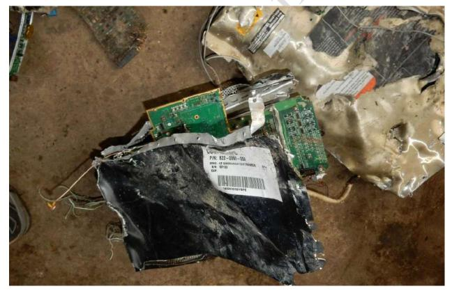
Fig. 17. The HF radio set switching unit fragments
