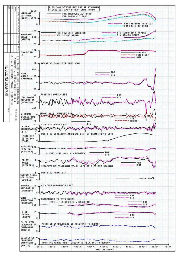
Fig. 47. The results of the engineering simulation (the lateral and directional channels)
