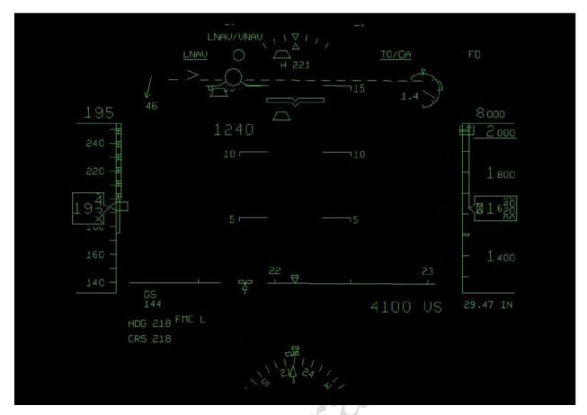
Fig. 65. The HUD reconstructed image at the point of time of 00:41:03 (the pitch local maximum ≈14°)
