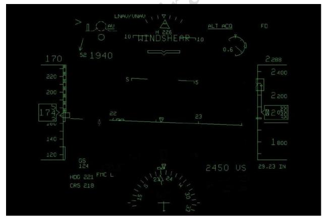
Fig. 59. The HUD reconstructed image at the point of time of 22:42:27.5 (the first press on the stabilizer trim switches)
