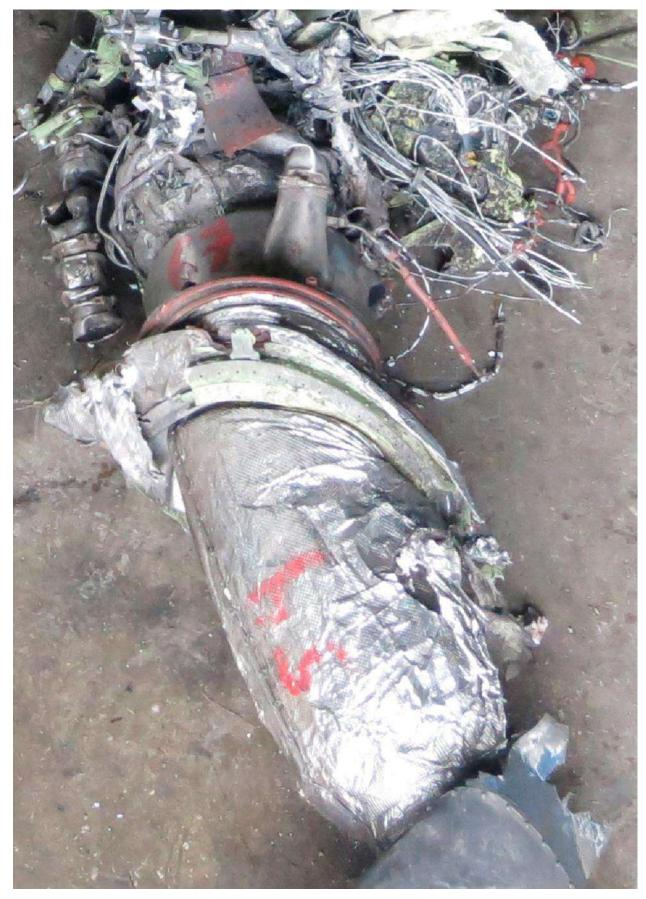
Fig. 14. The APU fragment with the exhaust duct and the fuselage tailcone
