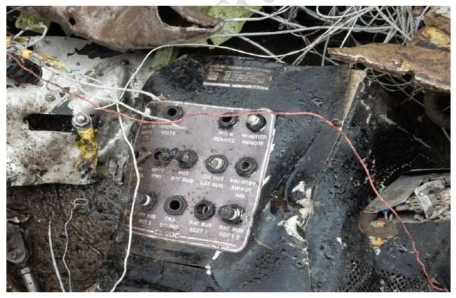
Fig. 19. The standby power control unit
