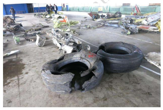
Fig. 10. The elements of the left main landing gear leg
