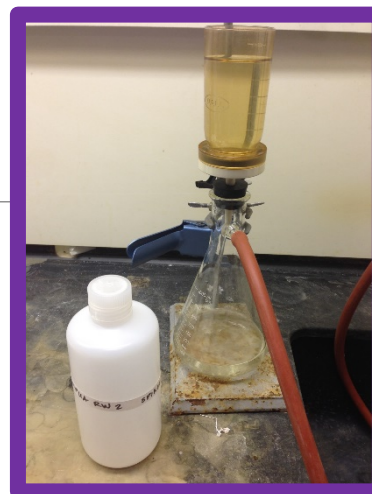
Filter water samples with pre combusted GF/F glass fiber filter
