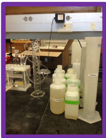
Collect water in 1 L HDPE bottles; Pour 500 ml of sample into graduated cylinders for volume measurement
