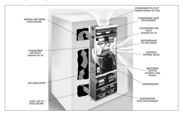
Kooltronic Air Conditioners are required when the equipment operating temperature must be kept near or lower than the ambient room temperature, and/or the cabinet must be sealed from dust, fumes, oil, corrosives and other contaminants. This Air Conditioner utilizes a "Closed-Loop Cooling System" to ensure optimum performance of the installed components.
