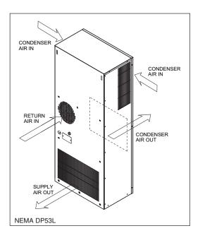
Any enclosure moisture accumulated on the evaporator coil is collected in the condensate tray and removed through the drain tube.
