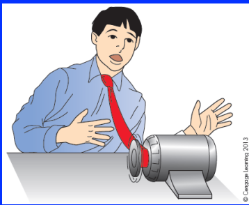
Figure 4-26 SAFETY PRECAUTION: Never wear a necktie or loose clothing when using or working around rotating equipment
