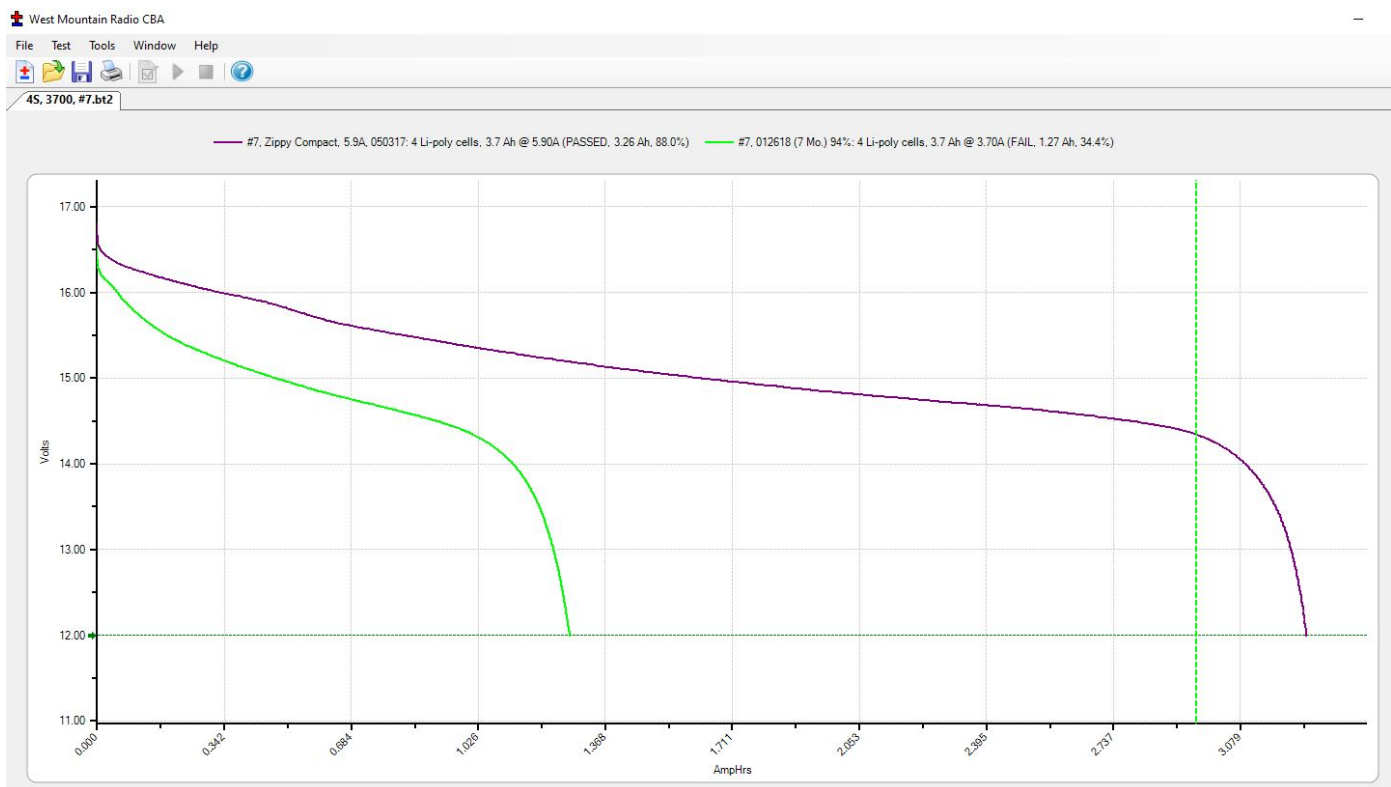
Chart 1. CBA test - Amp hour decay under constant current (5.9A load).
