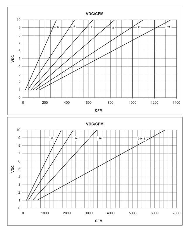
**Note:** This data is valid for the specific airflow sensor tubing size and lengths as shown on the wiring diagram. Readings will vary if different tubing size and lengths are used.
