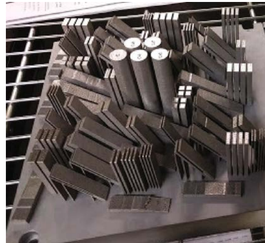
Fig. 2: (a) Schematic of the build plate, (b) photograph of full build plate and (c) schematic of the fully machined tensile sample
