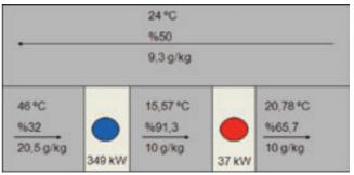
Design Values for a 100% Fresh Air Air Handling Unit without Heat Recovery
