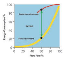
reduce power consumption; however none of these are as efficient as using flow control adjustment with frequency convector for power economy. For example, Start/Stop control, the increased number of starts and shut downs cause much higher mechanical tension and pressure increases resulting from fluctuations in the power source. The adjoining figure compares the power consumption of flow control with frequency converter and that of reducing power by damper.
