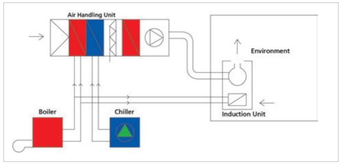
Water-Air System Schematic
