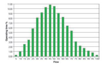
Air handling systems rarely need maximum design flow. Frequency converter alters the rpm of the fan motor in air handling units, adjusting the system air flow. In this way, while the required amount of fresh air is supplied, a high level of energy is saved. The following figure shows that 90% of the fan's operation occurs at 70% rpm.
