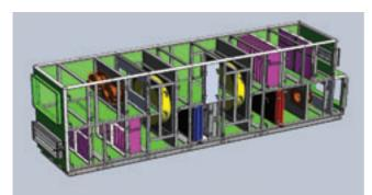
Double Rotor Air Handling Unit
