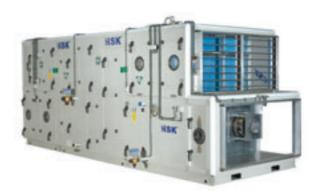
Interior and exterior surface material: Interior and exterior surface sheets have been manufactured from galvanized steel sheet. The exterior sheet surface is coated with 5  $\mu$  epoxy prime coat, a 20  $\mu$  polyester furnace paint top coat with colour code RAL 7035 and plastic film over the paint. Interior and exterior sheet thicknesses can be selected within the range 0.8 - 1.2 mm depending on requirements and place of use.
