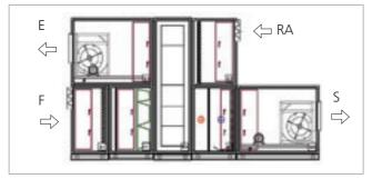
Air handling unit with rotor-type heat recovery is shown on Figure 5.
