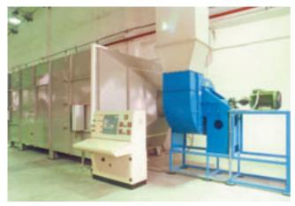
"Air Handling Unit Testing and Performance Measurement Room"
