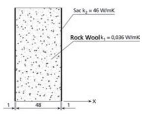
For example, we can calculate the heat conduction value by calculating heat conduction by taking the interior unit panel temperature as 17°C, the ambient temperature as 32°C for a surface area of 60 m<sup>2</sup>.
