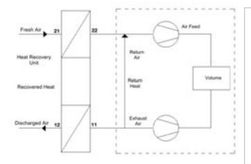
structure of the heat recovery unit. Heat recovery units can be divided in 2 general categories:
