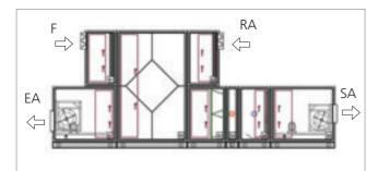
Air handling unit with heat recovery is shown on Figure 4. Heat recovery unit [S2] supplies the intake heat from the exhaust air to the fresh air and considerably increases the system efficiency.
