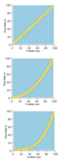
The most important point in terms of energy economy is that power consumption is proportional to the third power of fan rpm. This means that a drop in rpm will provide a significant reduction in energy consumption. Consequently, as seen in the figures as well, the power expended to bring the air flow to 75% is 40% of the energy of the motor operating at full speed.
