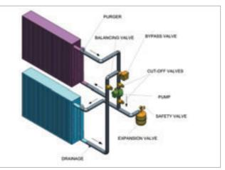
The enclosed circulation system allows the process to occur even when the outdoor air and exhaust air are at long distances to each other. Air currents do not have to come together, but additional energy to facilitate the circuit is needed. This is the electrical power required to operate the pump that facilitates the circuit. The amount of recovered heat can be easily regulated by controlling the flow of wa-
