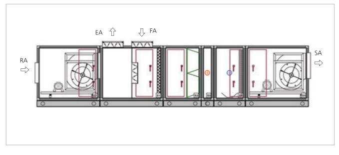
The design in Figure 3 is an air handling unit operating with mixed air. S1 in this figure shows the mixing chamber. This chamber determines how much of the intake air from the system is to be exhausted and how much to be added to the mixed air by working together with the dampers on it. These dampers can be controlled through servo motors governed by the automation system upon request. This allows comfort conditions to be ensured through minimum energy savings.
