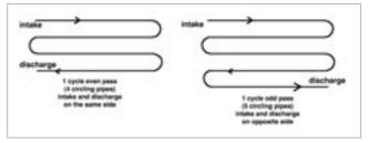
Figure 3.4. Intake - Discharge Directions According to Odd or Even Numbered Passes in Water Side Coil
