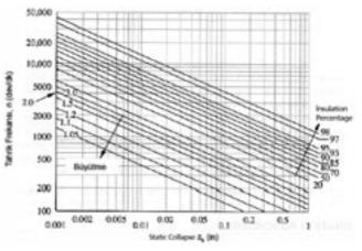
Figure 1- Variation of insulation efficiency with static collapse and frequency
