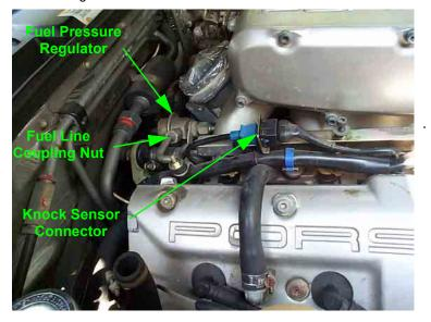
FIGURE 5 Right-Side Fuel, and Electrical Connections
