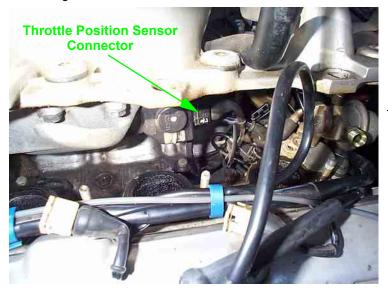
FIGURE 14 Throttle Position Sensor
