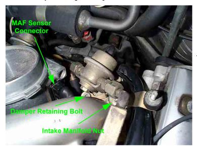
FIGURE 8 Rear Fuel Damper and MAF Sensor
