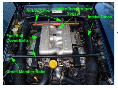
FIGURE 1 GT Engine Compartment 4
