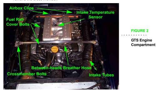
c. On GTS models remove the breather hose that connects to the front of the left and right cam covers. *See Figure 2.*
