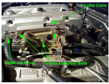
FIGURE 3 Throttle Cable Assembly
