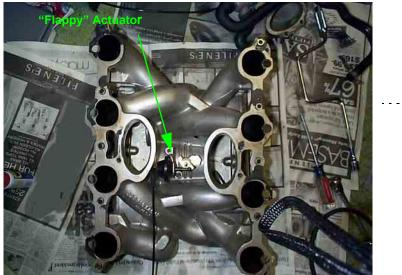
**FIGURE 17** \_ \_ \_ . "Flappy" Actuator
