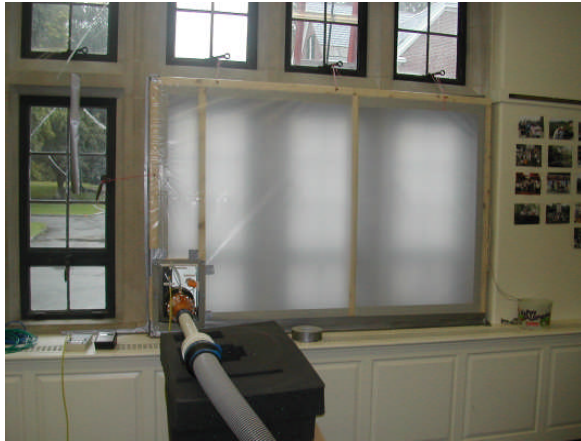
Photo 1 – Test chamber on window specimen
