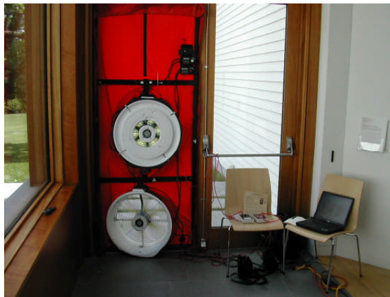
Photo 4 – Dual fan blower door used for whole-building airtightness test
