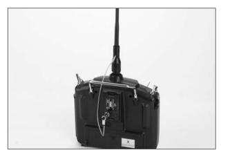
Turn on your transmitter. The LED on the back of the module should come 5. on after a few seconds. If not check to be sure the transmitter is in PPM modulation mode (Step 3 in preparing the transmitter above).
