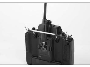
Turn on your transmitter. The LED on the back of the module should come on after a few seconds. If not check to be sure the transmitter is in PPM modulation mode (Step 3 in preparing the transmitter above).
