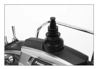
Antenna Adapter installed
