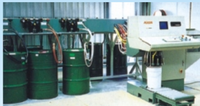
An ink pumping and mixing plant at Amcor Packaging in Australia using Blagdon 15 moulded pumps.
