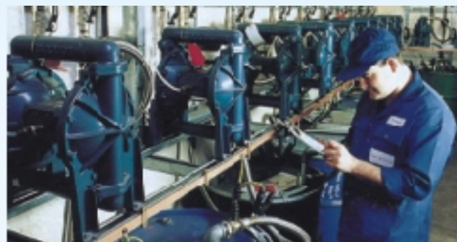
Fully automated Rexson ink manufacturing plant. Blagdon 25 metallic pumps are used for mixing and recirculation.
