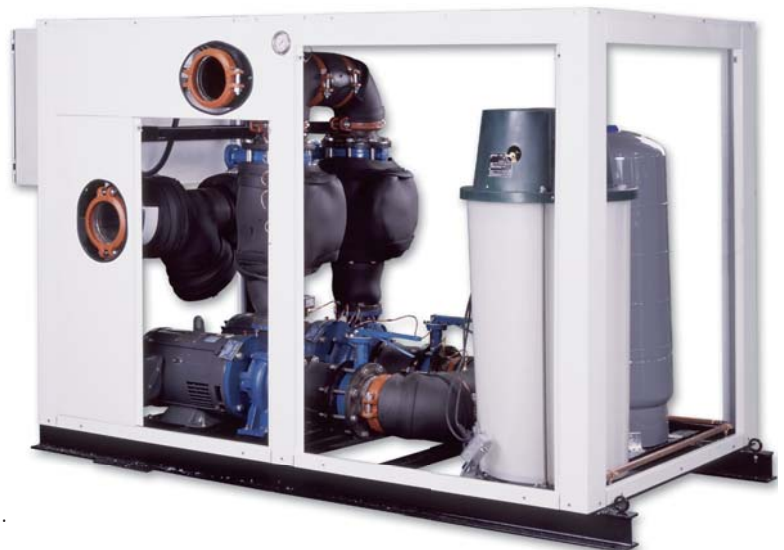
Water Manifolds are schedule 40 steel pipe. Modules are attached using roll-groove couplings. Optional isolation valves.
