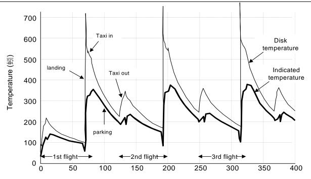
Figure 7 - Example of brake temperature profile achieved over given route data (Aircraft not equipped with brake cooling fans)
