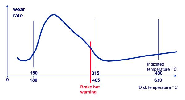
Figure 3 - Carbon Wear vs. Brake Temperature according to HONEYWELL-ALS (A330 / A340)
