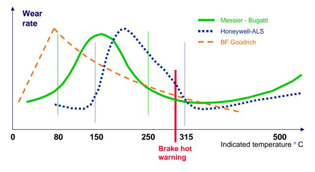
Figure 6 - Carbon Wear vs. Indicated Brake Temperature Messier-Bugatti, Honeywell-ALS and BF Goodrich
