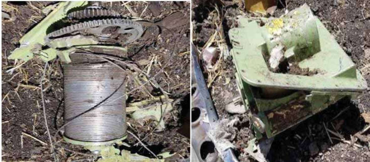
FIGURE 50:AFT CABLE DRUM
