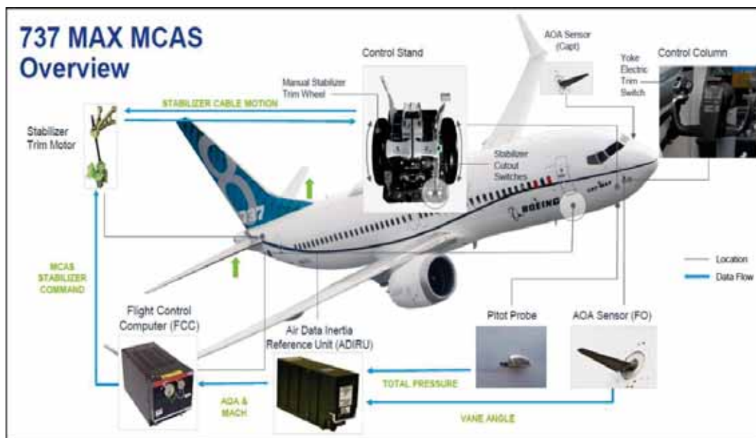
FIGURE 13: DIAGRAM SHOWING THE COMPONENTS OF MCAS 11
