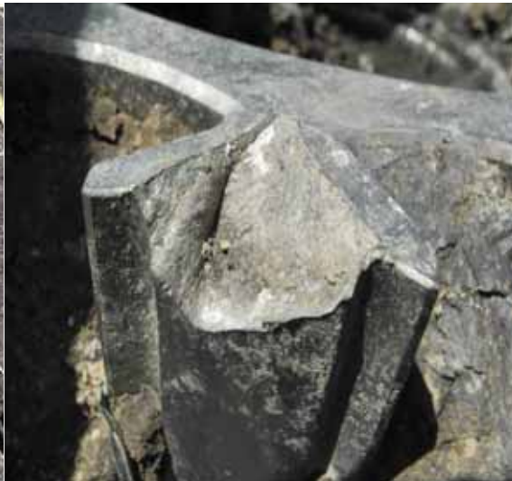
FIGURE 39: R/H ENGINE - S/N 602695 - RETENTION LUGS - FRACTURED
