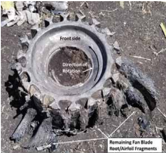
FIGURE 38: R/H ENGINE - S/N 602695 – FAN DISK
