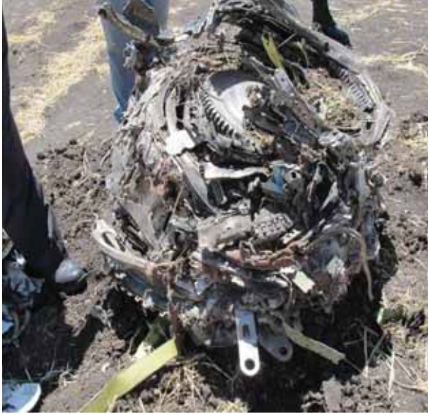
FIGURE 36: R/H ENGINE - S/N 602695 – CORE
