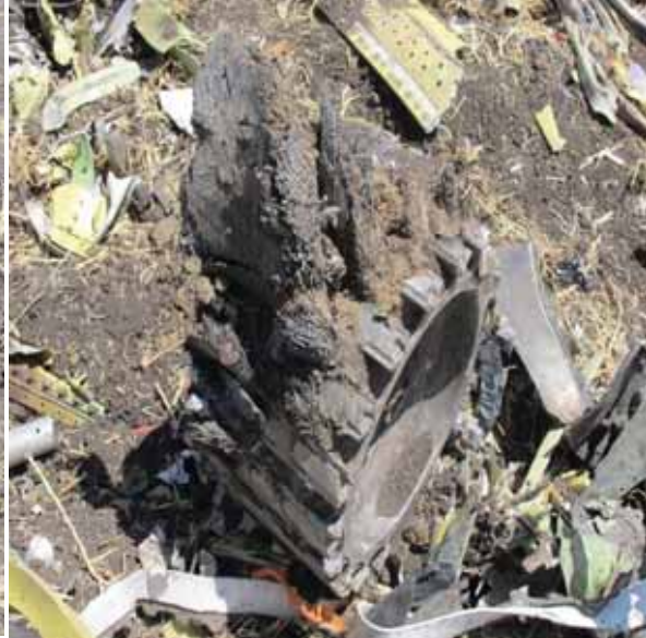
FIGURE 37: - R/H ENGINE - S/N 602695 – FAN DISK
