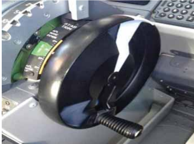
FIGURE 12: THE TRIM WHEEL, WITH THE HANDLE EXTENDED
