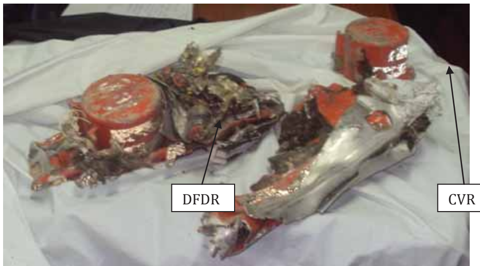
FIGURE 24: DFDR AND CVR AS DISCOVERED ON THE ACCIDENT SITE.
